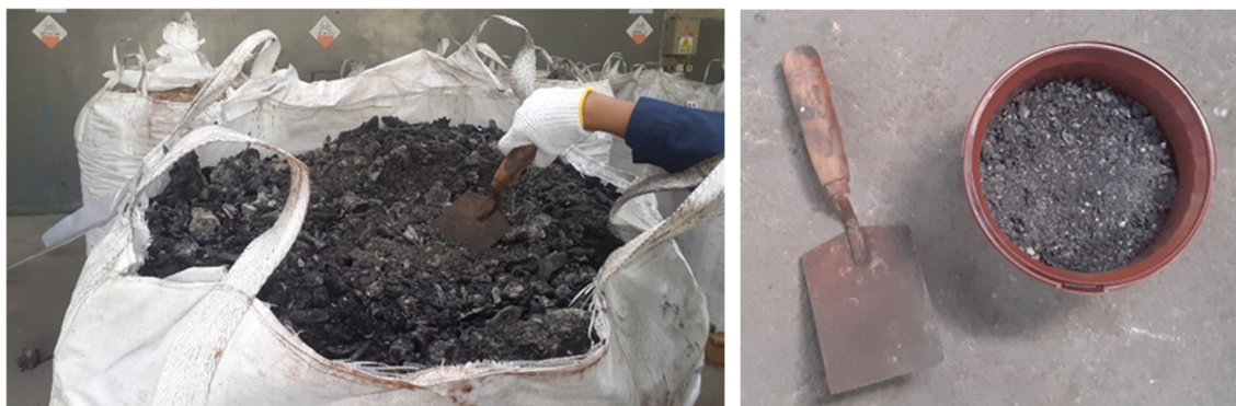
Fig. 1. (a) Residues from burning infectious waste, (b) Residues from burning infectious waste that has been filtered
