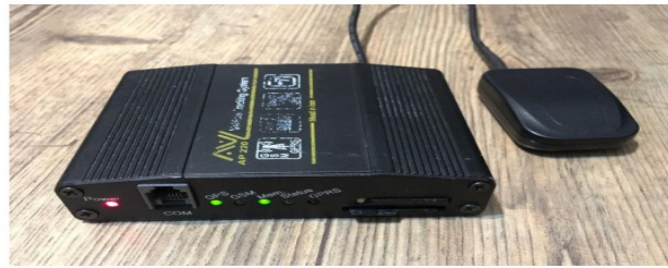
Fig. 1. GPS device used for recording the vehicle's speed and acceleration data on a second-by-second basis
