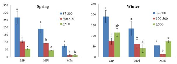
**Figure 3.** The numbers of microplastics (MP), synthetic microfibers (MFi) and plastic microparticles (MPa) in different size classes in the treated effluent from the Sari wastewater treatment plant in Iran, sampled in spring (left) and winter (right) ( $\pm$ SE, n=3). Bars with the same letter do not differ significantly between size classes.
