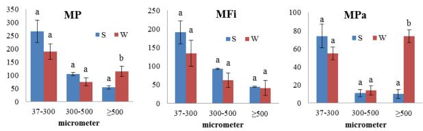
**Figure 2.** The numbers of microplastics (MP), synthetic microfibers (MFi) and plastic microparticles (MPa) in different size classes in treated effluent from the Sari wastewater treatment plant in Iran in Spring (S) and Winter (W). ( $\pm$ SE, n=3). Bars with the same letter do not differ significantly between spring and winter.
