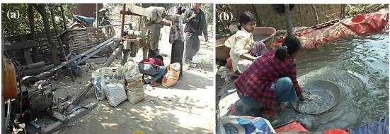
**Fig 2.** Ore crushing (a) and screening (b) process occurred in the yard. Ore crushing equipment, which is assembled from simple agricultural equipment, and reservoirs are distributed in courtyards with limited space. Among the people we interacted with, all family members who were able to work participated in ASGM activity for a household.
