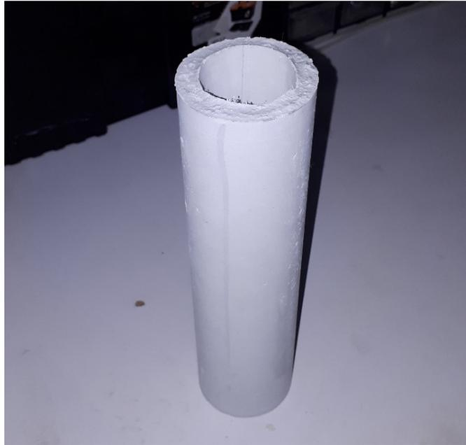
**Fig. 1.** photocatalytic cement composite specimen as a fixed bed
