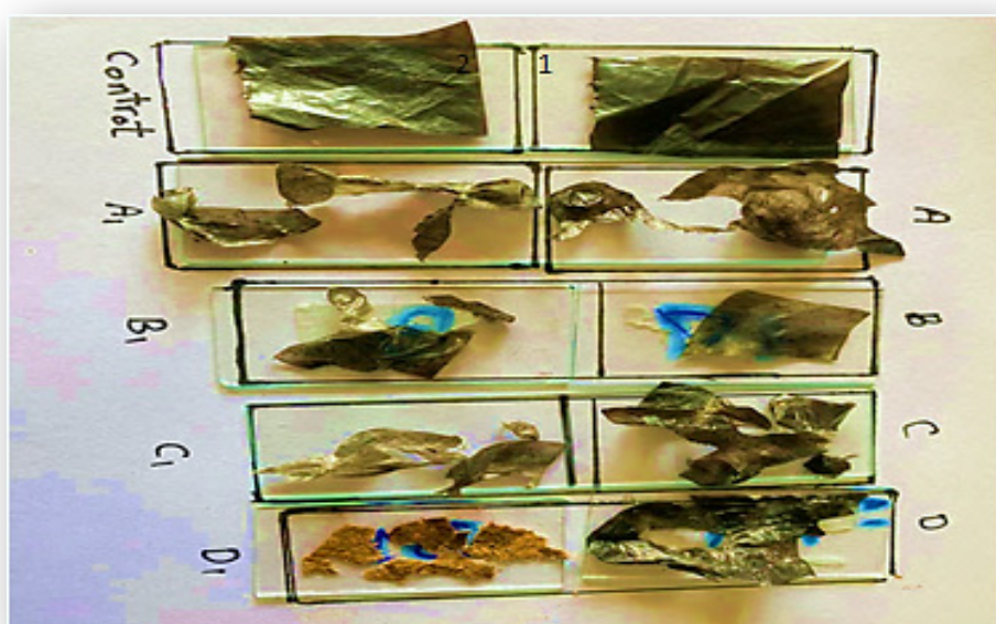
Fig. 4. Morphology of plastic film. Control strips before exposure – control 2: strips after exposure-A:(A, A1) in soil without additives after degradation; (B, B1) soil with addition of rice husk after degradation; (C, C1) soil with addition of peatmos after degradation; (D, D1) soil with addition of organic fertilizers after degradation
