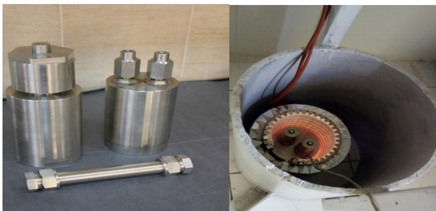
Fig. 1. High-pressure batch type reactor with electrical furnace
