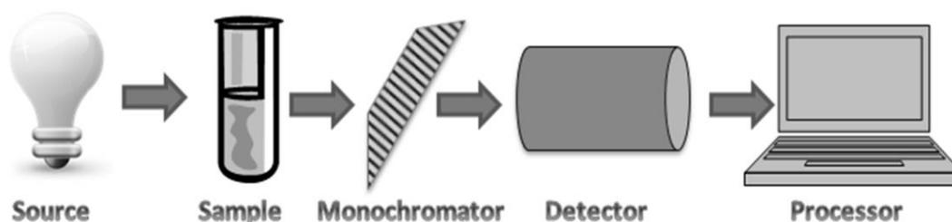
**Fig. 2. Basic illustration of atomic absorption spectrometer.**
