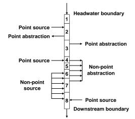
Fig 4. QUAL2Kw model subdivision for river without branches
