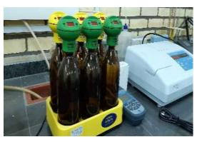
Fig 2B. Device for measuring BOD
