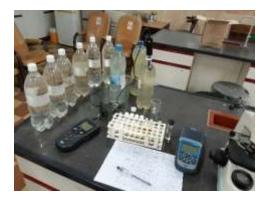
Fig 2A. Device for measuring Dissolved oxygen
