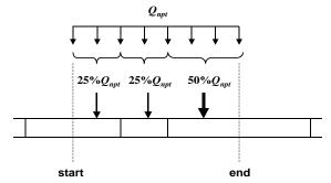
Fig 6. Way of considering non-point input sources to an element in the QUAL2Kw
