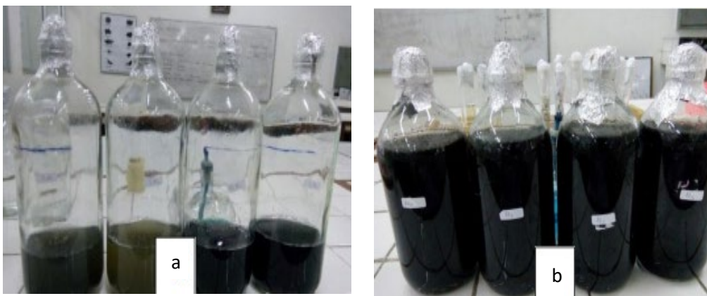
Fig. 2. SRB active suspension (a) before cultivation and (b) after cultivation
