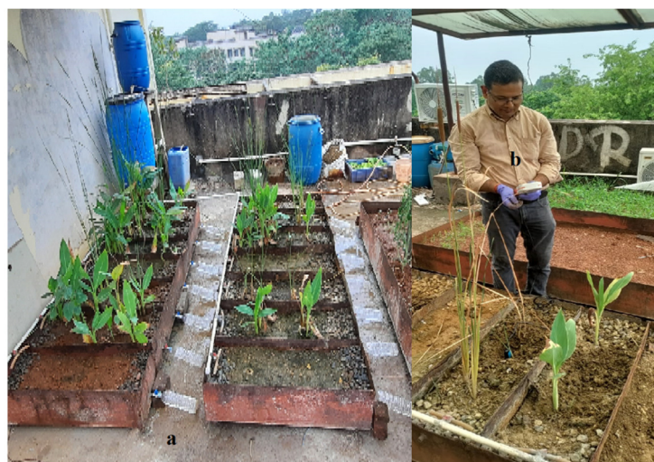
Fig. 2. Canna indica and Typha latifolia in various soil and aggregate media-type CWs (a) experimental setup (b) starting with plant density two
