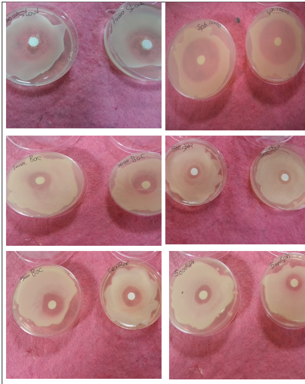
Fig. 6. the antibacterial activity of \text{CuFe}_2\text{O}_4 NPs in the different concentration(ppm) against different types of bacteria
