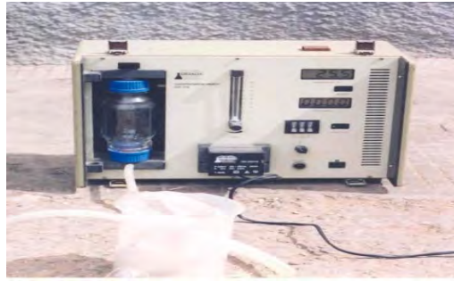
Fig. 3. Sampler for Sulphur and nitrogen compounds
