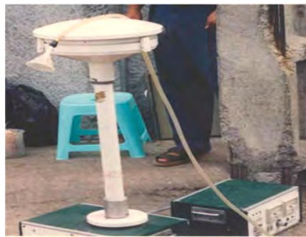
Fig. 5. High-volume sampler HVS
