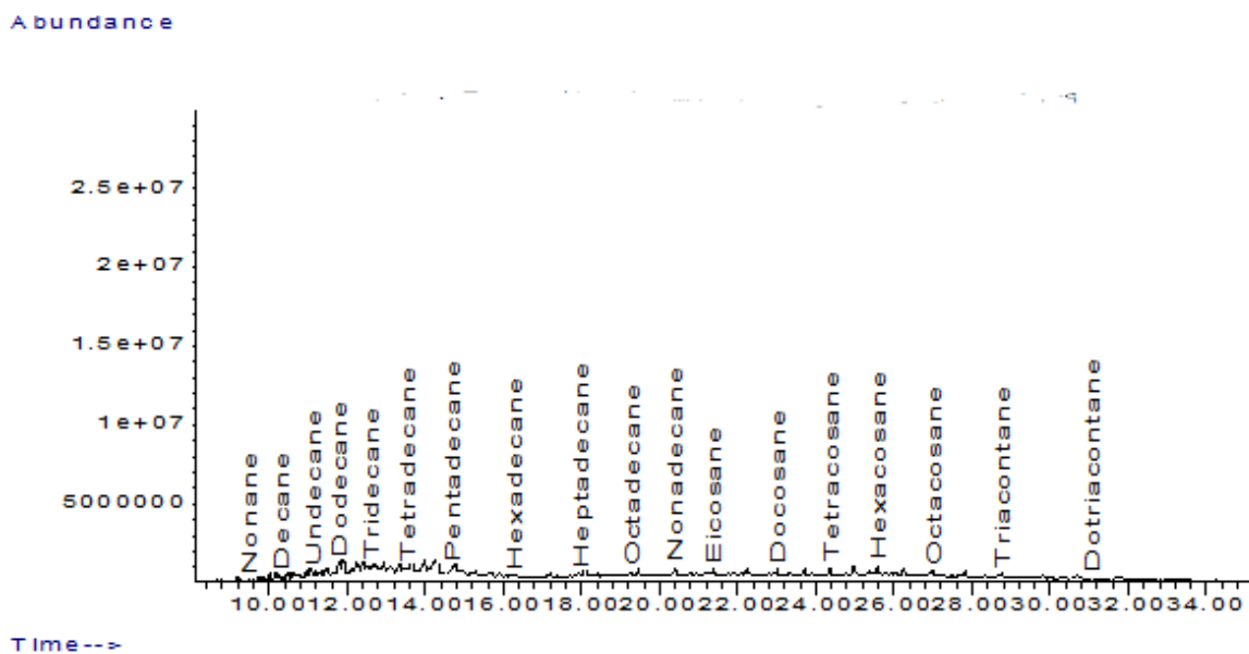
Fig. 6. Mass chromatogram of the degraded Extractable total Petroleum Hydrocarbon in the crude oil samples by P. aeruginosa strain KUD2
