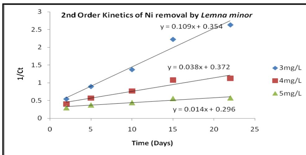
Fig. 5. Second Order Removal kinetics of Ni removal by *Lemna minor*
