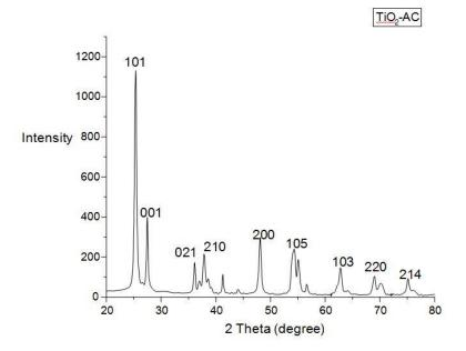
Fig. 3. XRD patterns of TiO<sub>2</sub>/Activated carbon nanocomposite
