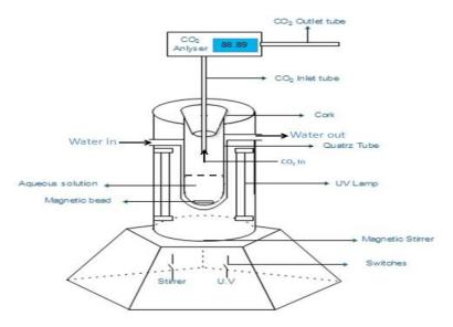
Fig. 2. Line diagram of photochemical reactor
