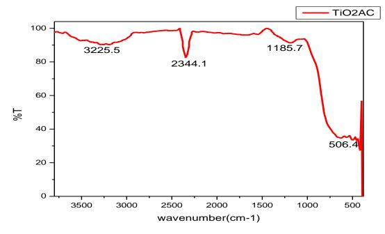
Fig. 5. FT-IR spectra of TiO<sub>2</sub>/Activated carbon nanocomposite
