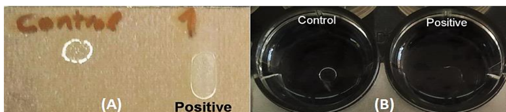
Fig. 3. Biosurfactant production assay by glass slide test (A) and drop collapsed test (B)
