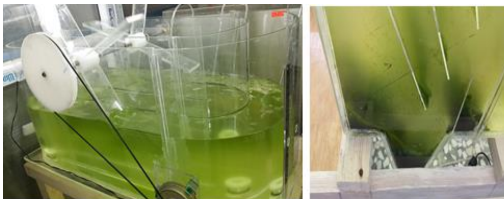
Fig. 2. Left: open raceway pond; Right: sedimentation zone
