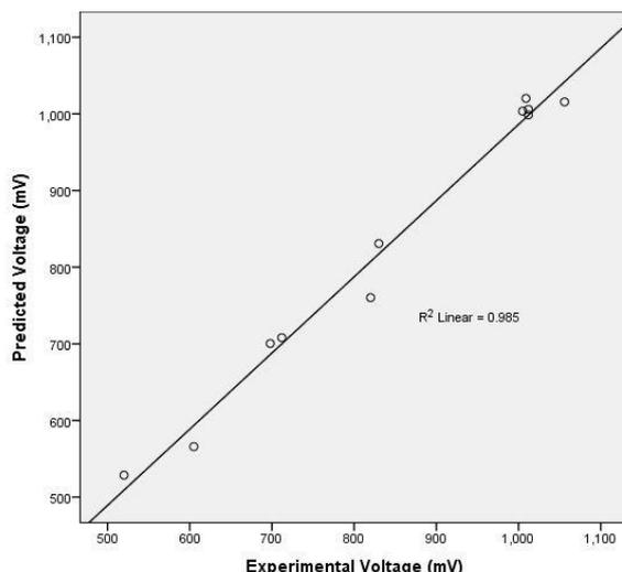
Fig. 9. Maximum experimental voltage with the predicates voltage of MFC.
