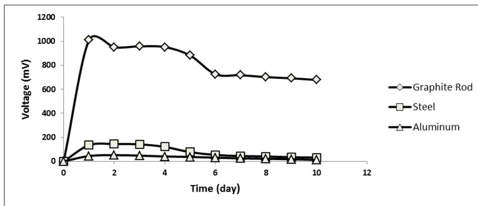
Fig. 6. Voltage generation (mV) with time (days) by different electrode type
