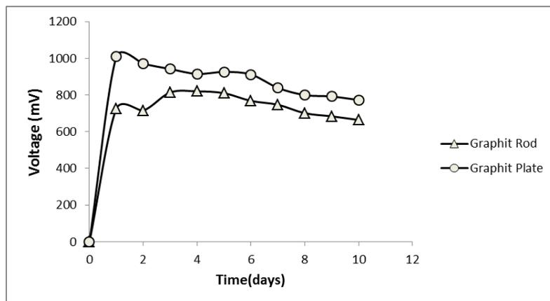
**Fig. 7. Voltage (mV) of graphite rod and graphite plate**
