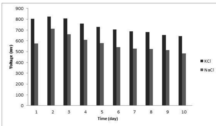
**Fig. 3.** Voltage (mV), generated in MFC for 1M KCl and 1M NaCl, with respect to time (days).
