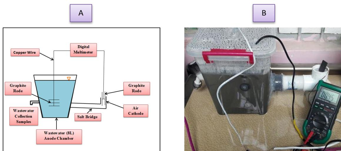
**Fig. 1. (A) Schematic diagram of MFC. (B) MFC photo.**
