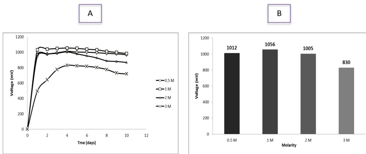
**Fig. 4.** (A) Voltage production (mV) with time (days) (B) Maximum voltage, obtained at different molar concentration
