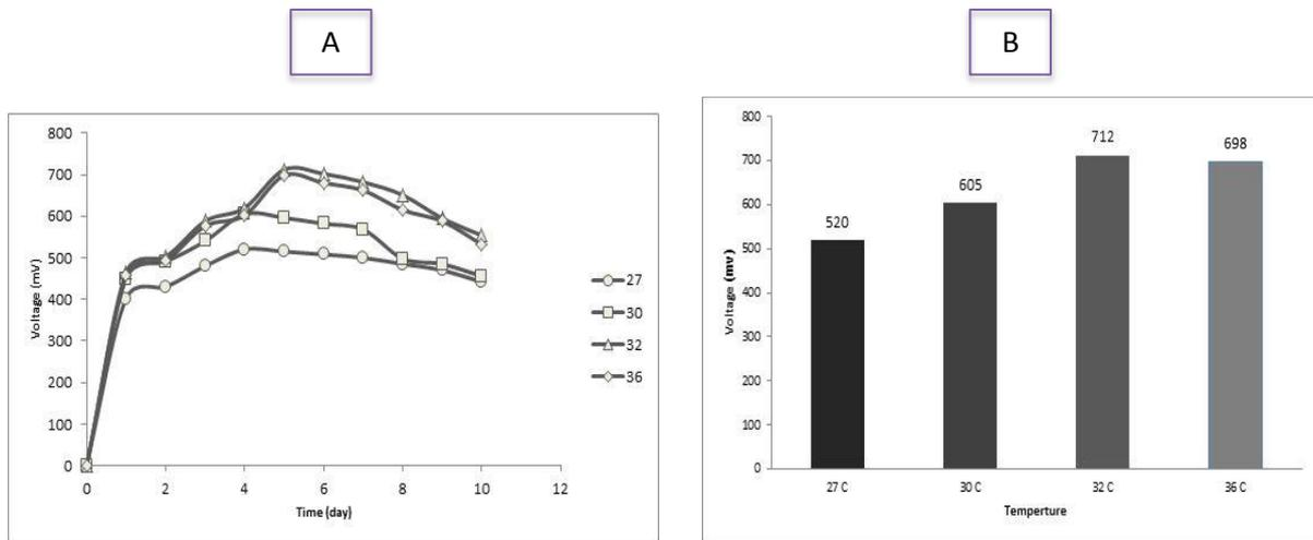
Fig. 5. (A) Voltage generation (mV) with time (days) at different temperatures (B) Value of maximum voltage, obtained at different temperatures
