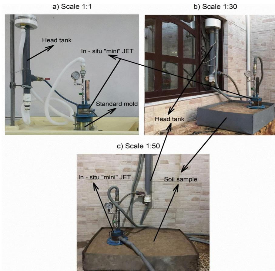
**Fig.1. Illustration of performing JET setup at different compacted soil scaling ratios: a) 1:1 scale, b) 1:30 scale, and c) 1:50 scale**
