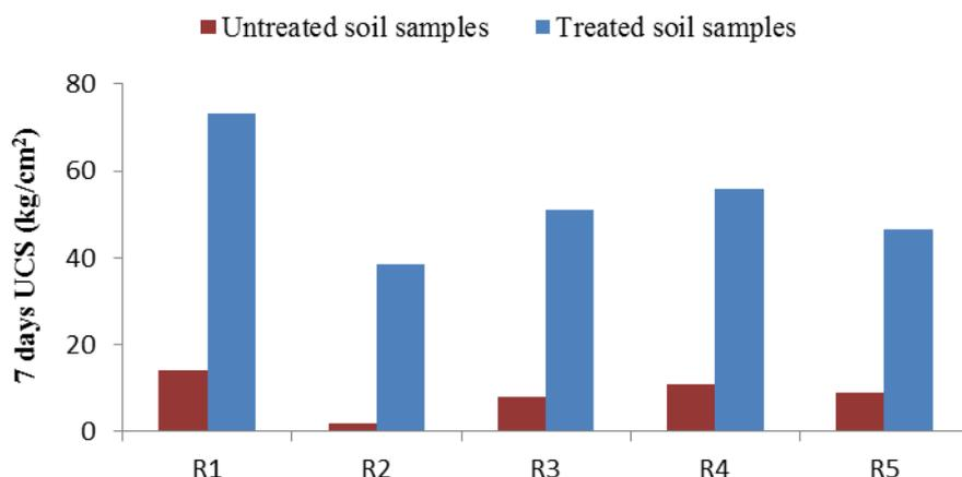
**Fig. 2. Variation of UCS in treated and untreated soil samples**
