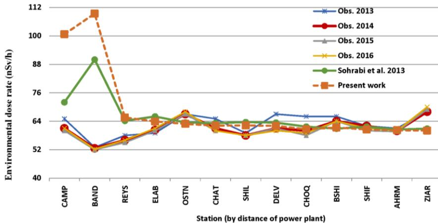
**Fig. 7. Environmental gamma dose rates (nSv/hr) (The power plant monitoring network observational data and results of Sohrabi et al. (2013) are present)**
