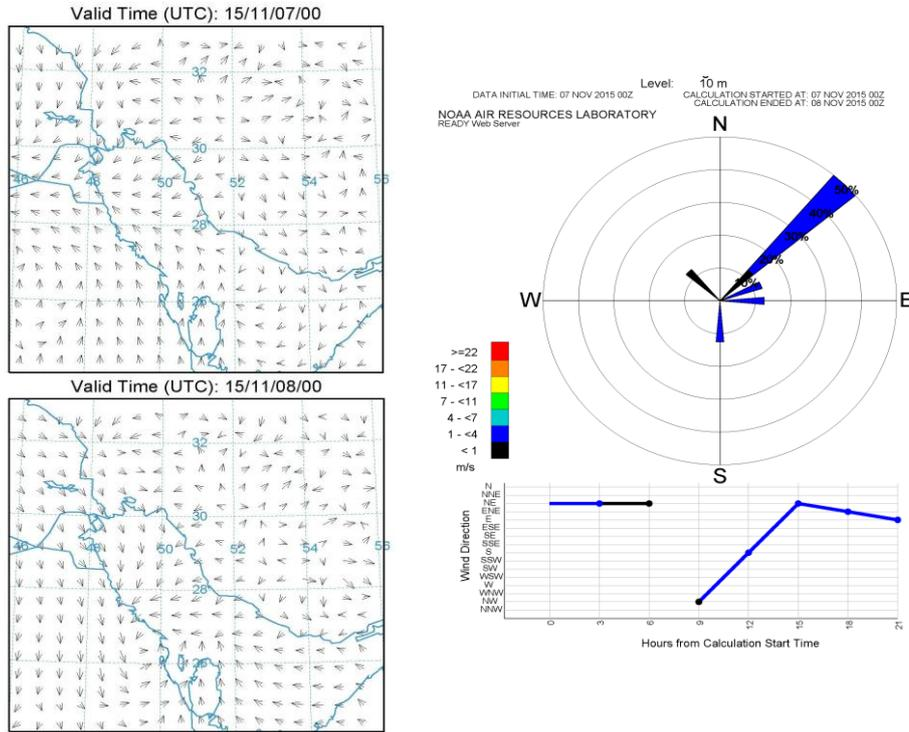
Fig. 12. Wind field, simulated by WRF model, and wind rose diagram (right), on November 7, 2015
