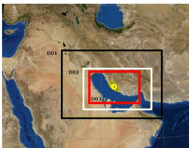
**Fig. 2. Computational domains of WRF model, used in this research**
