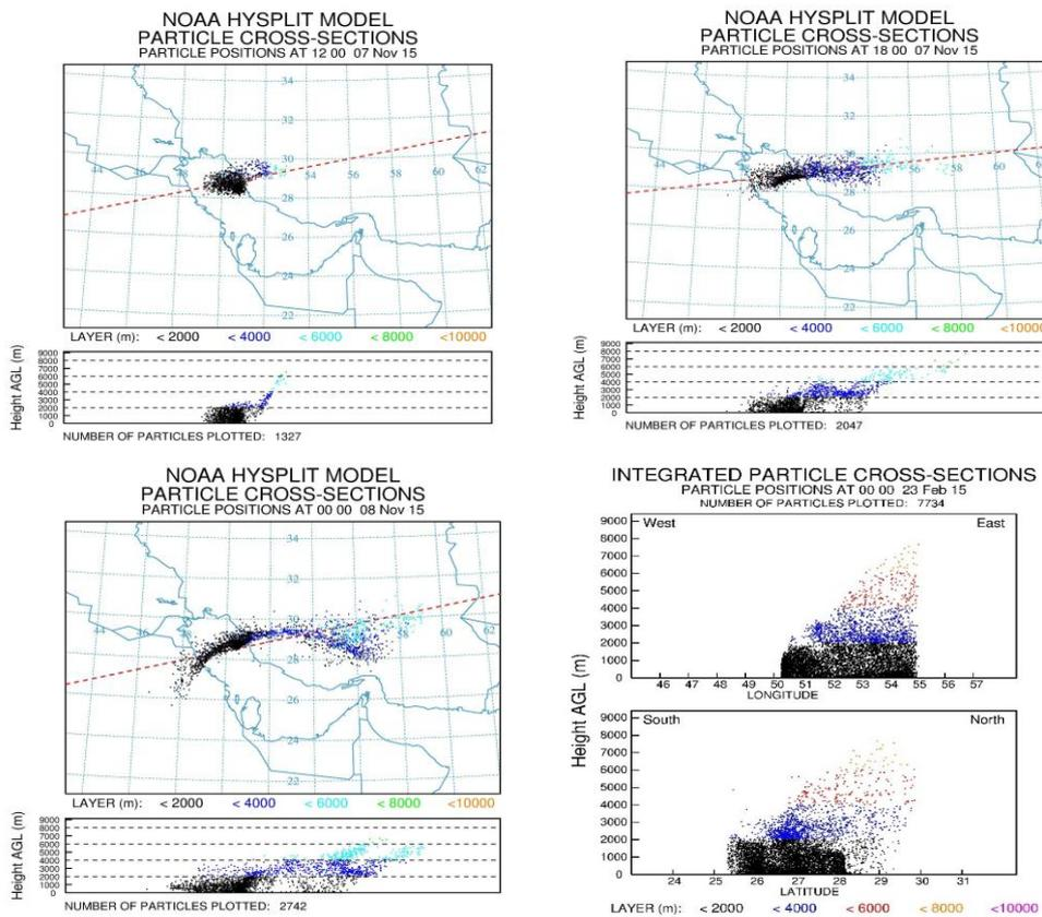
Fig.13. Time evolution of simulated particles plume by WRF-HYSPLIT, on November 7, 2015
