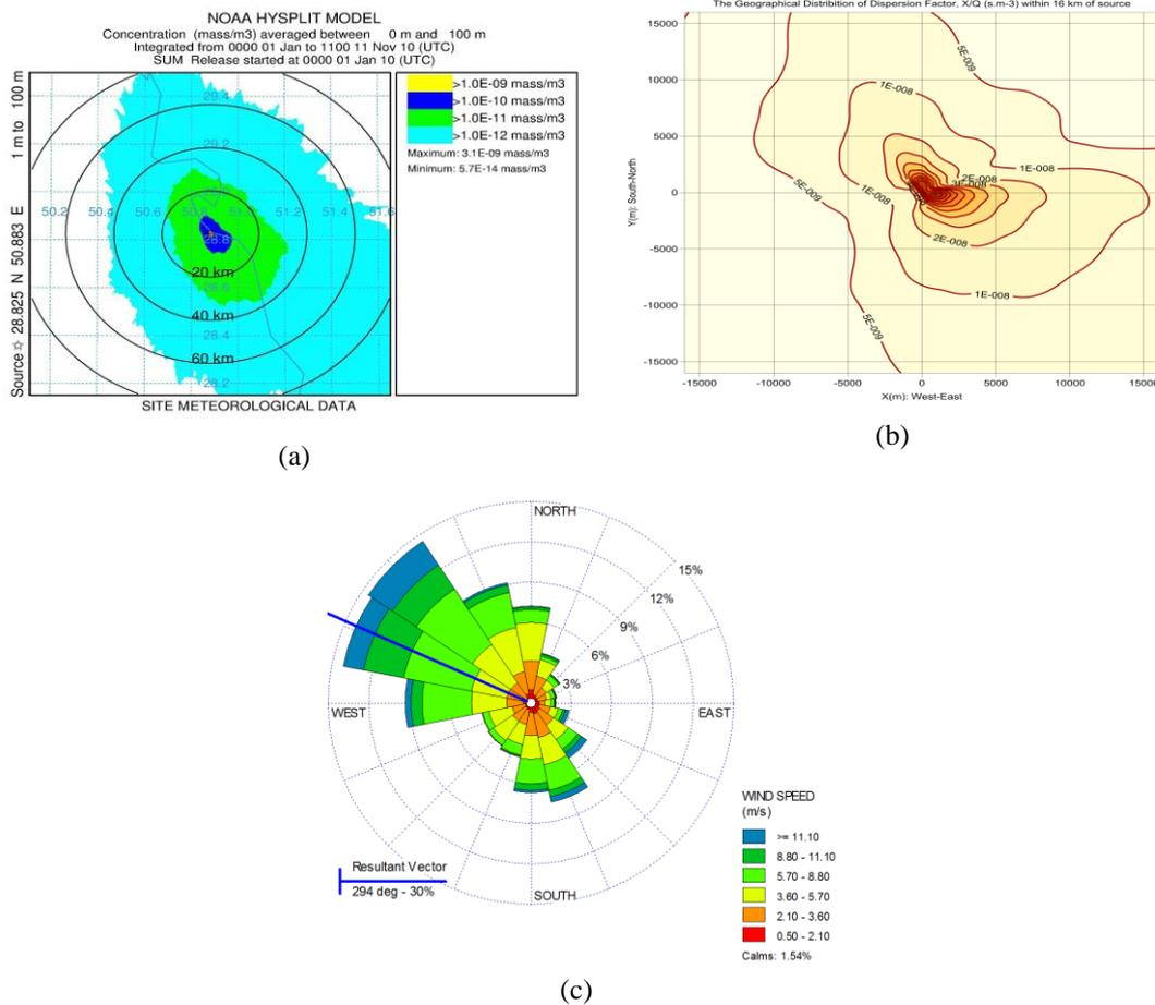
**Fig. 5. The annual atmospheric dispersion pattern, (a) the present work, (b) 2010 given in ER, and (c) wind rose for 2010**
