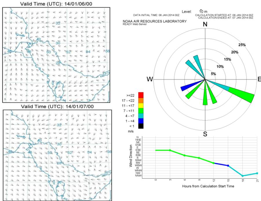
Fig. 8. Wind field, simulated by WRF model, and wind rose diagram (right), on January 6, 2014
