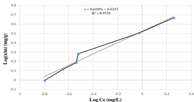
Fig. 13. Freundlich isotherm of nickel adsorption via  $\alpha$ -Fe<sub>2</sub>O<sub>3</sub> nanoparticles
