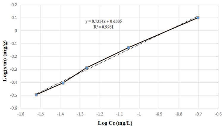
Fig. 15. Freundlich isotherm for cadmium adsorption via  $\alpha$ -Fe<sub>2</sub>O<sub>3</sub> nanoparticles
