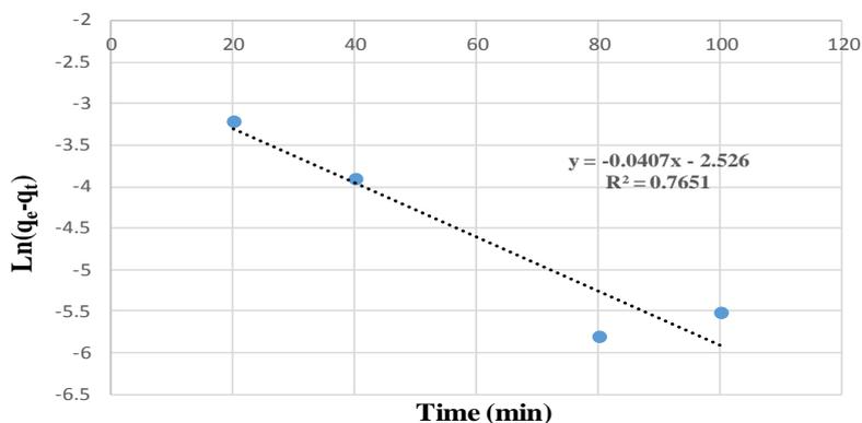
Fig. 11. Pseudo-first-order equation curve for cadmium adsorption via  $\alpha$ -Fe<sub>2</sub>O<sub>3</sub> nanoparticles
