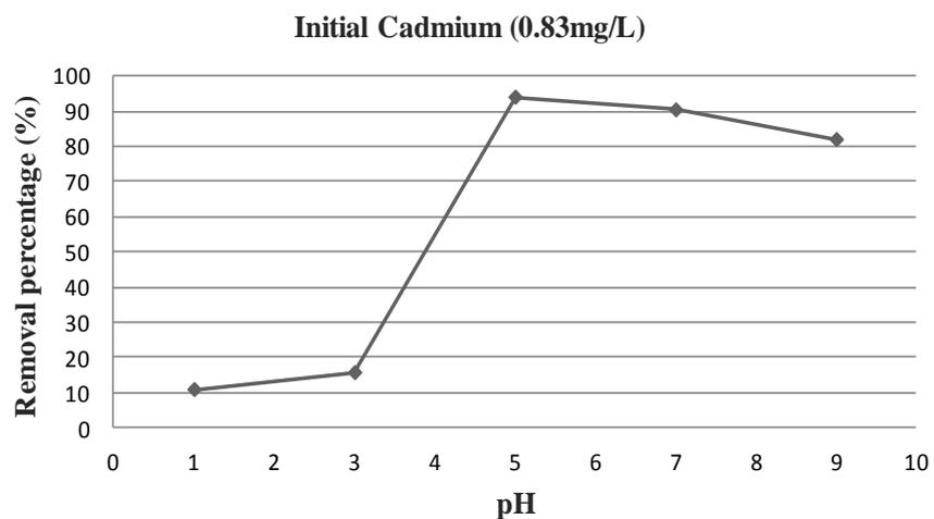
Fig. 4. the impact of pH on cadmium adsorption via magnetic  $\alpha$ -Fe<sub>2</sub>O<sub>3</sub> nanoparticles
