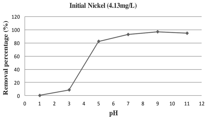
Fig. 3. The effect of pH on nickel adsorption via magnetic  $\alpha$ -Fe<sub>2</sub>O<sub>3</sub> nanoparticle
