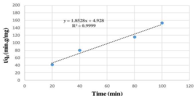
Fig. 12. Pseudo-second-order equation curve for cadmium adsorption via  $\alpha$ -Fe<sub>2</sub>O<sub>3</sub> nanoparticles
