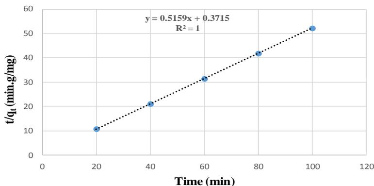
Fig. 10. Pseudo-second order equation curve for nickel adsorption via  $\alpha$ -Fe<sub>2</sub>O<sub>3</sub> nanoparticles
