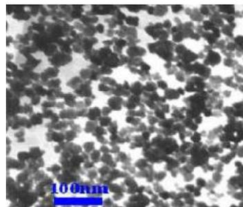
Fig. 1. The transmission electron microscopy of the magnetic nanoparticle  $\alpha$ -Fe<sub>2</sub>O<sub>3</sub> (TEM)
