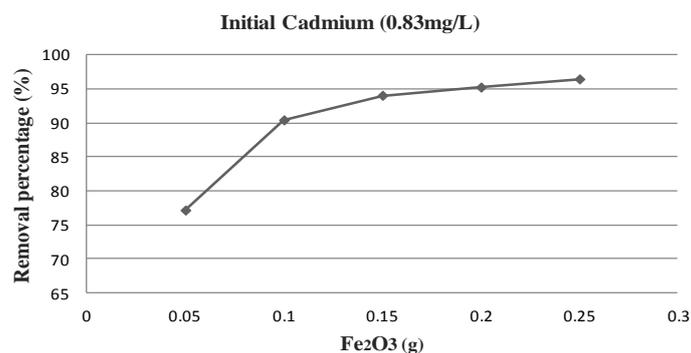
Fig. 6. Effect of amounts of  $\alpha$ -Fe<sub>2</sub>O<sub>3</sub> nanoparticle on cadmium adsorption
