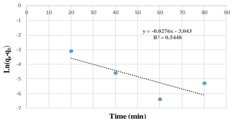
Fig. 9. Pseudo-first-order equation curve for nickel adsorption via  $\alpha$ -Fe<sub>2</sub>O<sub>3</sub> nanoparticles
