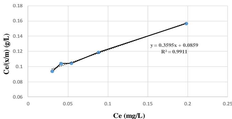
Fig. 16. Langmuir isotherm for cadmium adsorption via  $\alpha$ -Fe<sub>2</sub>O<sub>3</sub> nanoparticles
