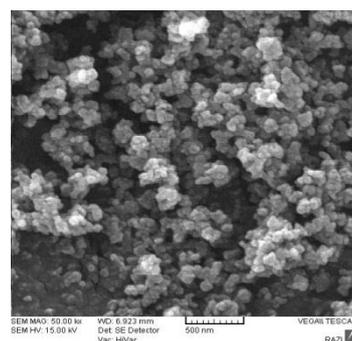
Fig. 2. The scanning electron microscopy of the magnetic nanoparticle  $\alpha$ -Fe<sub>2</sub>O<sub>3</sub> (SEM)
