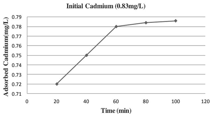
Fig. 8. Effect of time on cadmium adsorption via magnetic  $\alpha$ -Fe<sub>2</sub>O<sub>3</sub> nanoparticles
