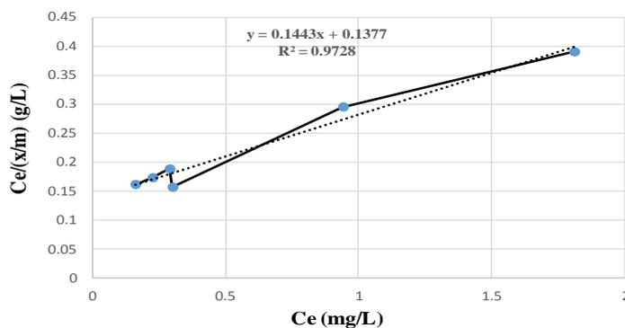
Fig. 14. Langmuir isotherm of nickel adsorption via  $\alpha$ -Fe<sub>2</sub>O<sub>3</sub> nanoparticles
