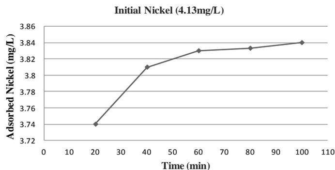
Fig. 7. Effect of time on nickel adsorption via magnetic  $\alpha$ -Fe<sub>2</sub>O<sub>3</sub> nanoparticles
