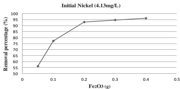
Fig. 5. Effect of  $\alpha$ -Fe<sub>2</sub>O<sub>3</sub> nanoparticle amounts on nickel adsorption
