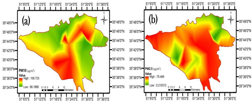
Fig. 5. Dispersion of (a) PM10, and (b) PM2.5 concentrations
