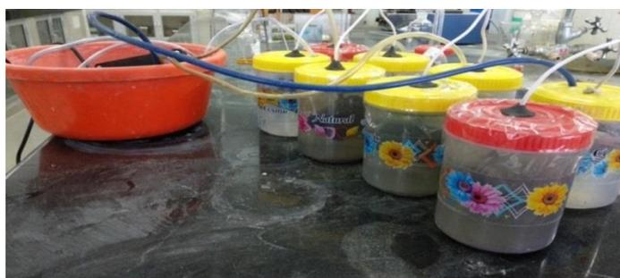
Fig. 1. An Experimental set up of microbial fuel cell with different catholyte
