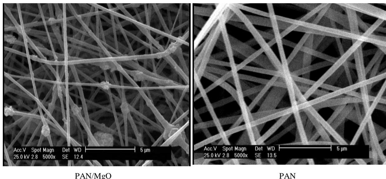
Fig. 2. SEM image of manufactured nanofibers
