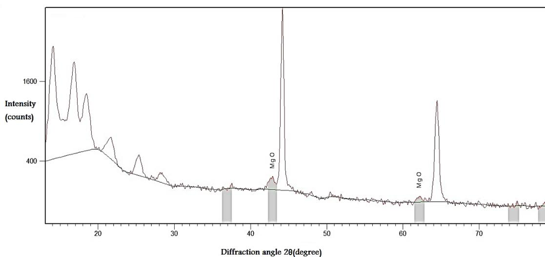
Fig. 5. X-ray diffraction Pattern of PAN/MgO nanofibrous filter
