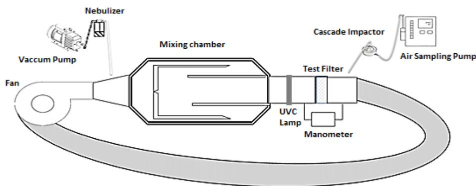
Fig. 1. Schematic design of filter test rig
