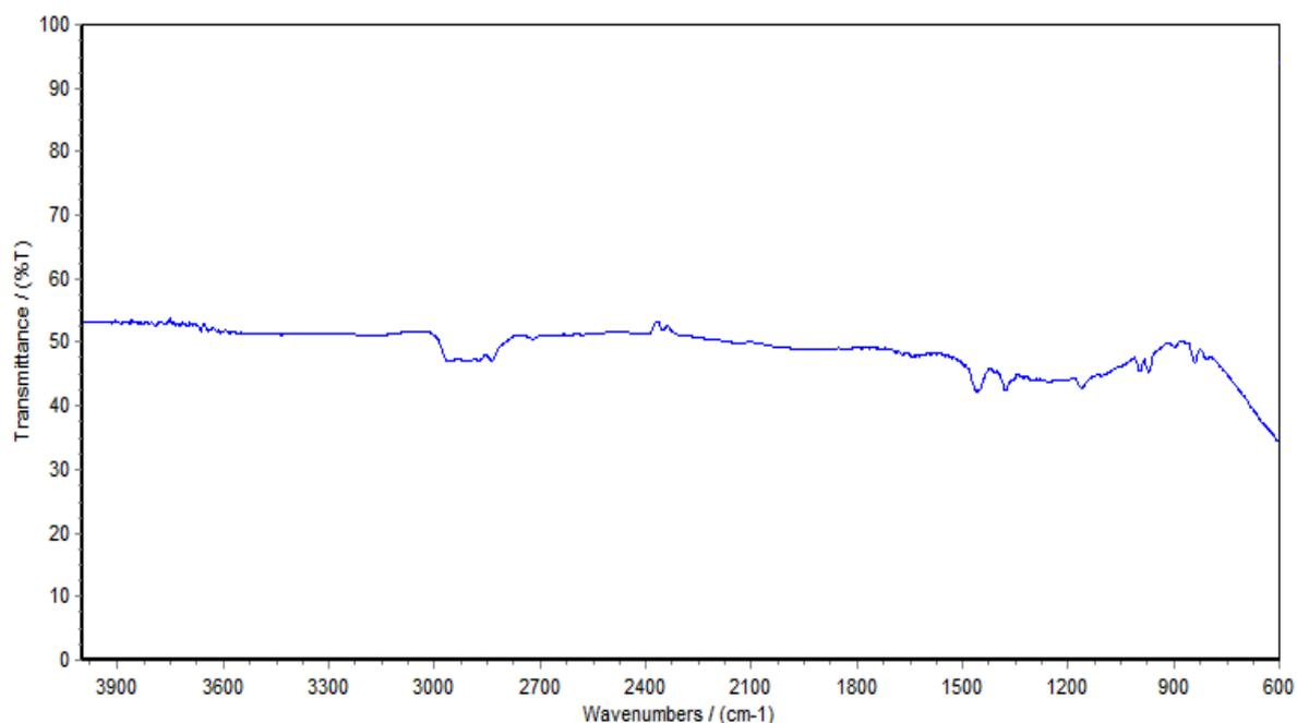
**Fig. 3. FTIR spectra of PAN nanofibers**
