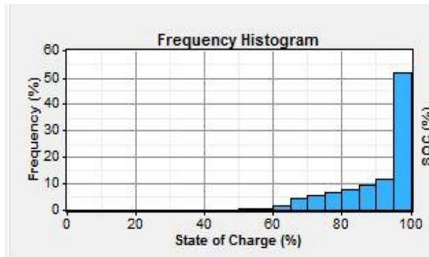
**Fig. 9. Frequency histogram for SOC of battery bank**
