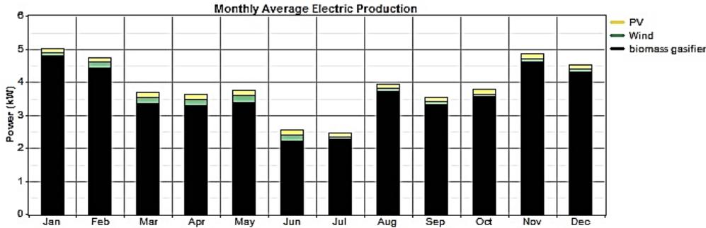
Fig. 6. Monthly average electricity generation from PV/Biomass/Wind/Battery hybrid system
