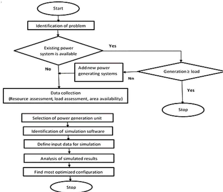
**Fig. 3. Flow chart of methodology used in hybrid system designing**
