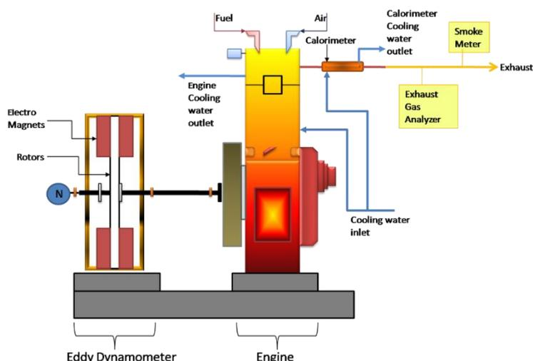
**Fig. 1. Schematic image of the engine set up.**
