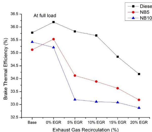
Fig. 2. Brake thermal efficiency vs exhaust gas recirculation at full load.
