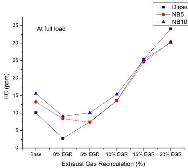
**Fig. 4. Hydrocarbon vs EGR at full load.**
