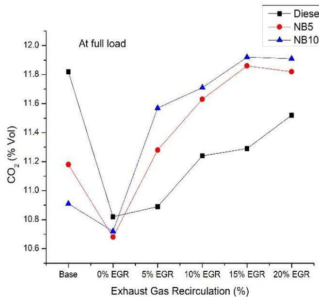
**Fig. 5. Carbon dioxide vs EGR at full load.**
