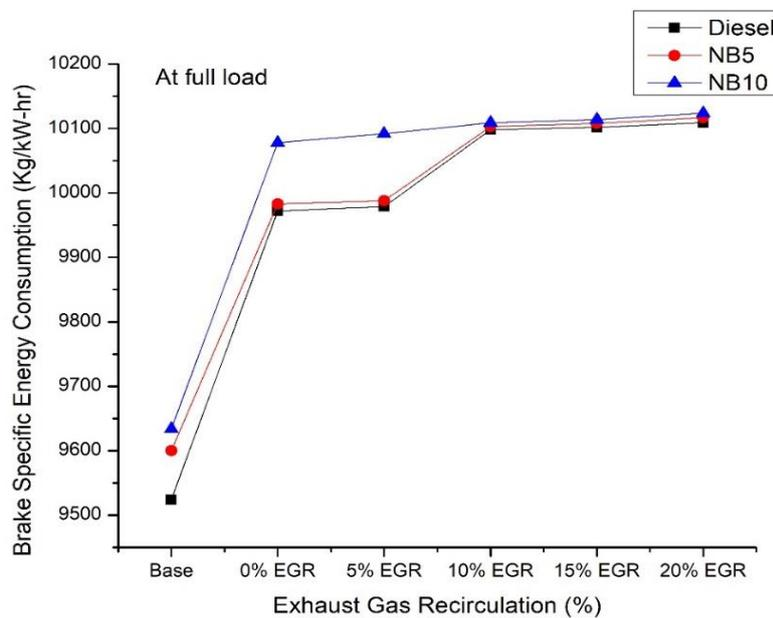
Fig. 3. Brake specific energy consumption vs exhaust gas recirculation at full load.
