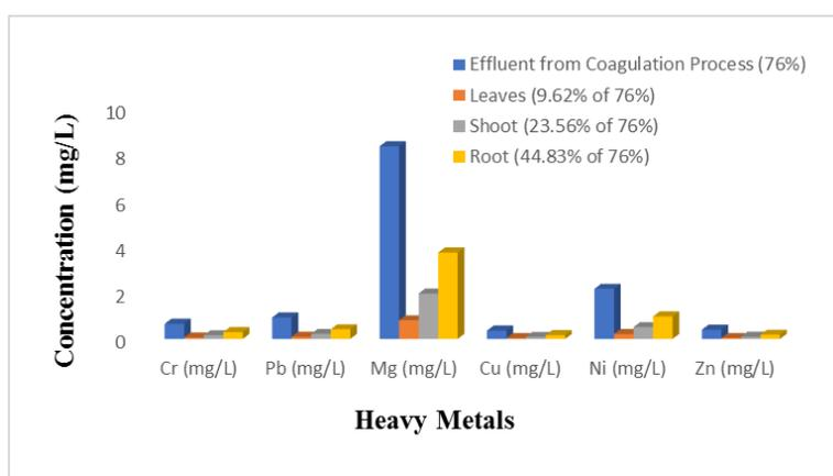
**Fig. 1. Heavy metal removal efficiency after coagulation-flocculation**
