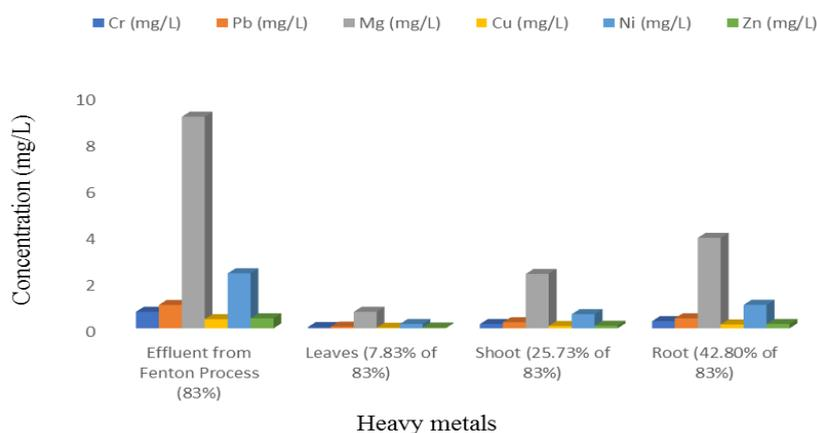
Fig. 2. Heavy metal removal efficiency after Fenton process
