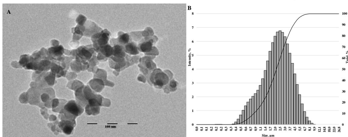
**Fig. 1. Transmission electron microscopic (TEM) image (A) and DLS size distribution of TiO<sub>2</sub>-NP (B) showing the aggregation pattern of TiO<sub>2</sub>-NP in seawater (24 h after sonication). Scale bar is 100 nm.**
