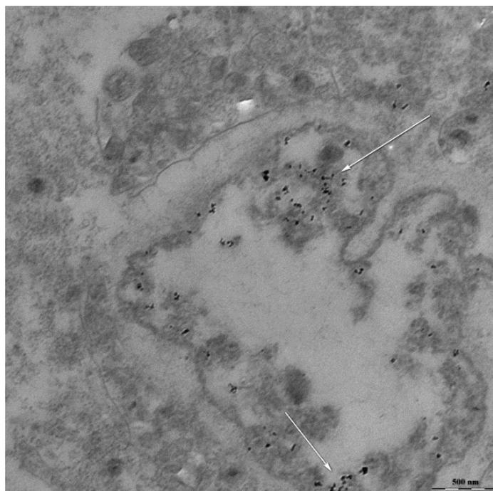
**Fig. 2.** Transmission electron microscopic observations for location of TiO<sub>2</sub>-NP in digestive gland of mussels after exposure to 1mg/l TiO<sub>2</sub>-NP for 10 days. Arrows point to a TiO<sub>2</sub>-NP. Scale bar is 500 nm.
