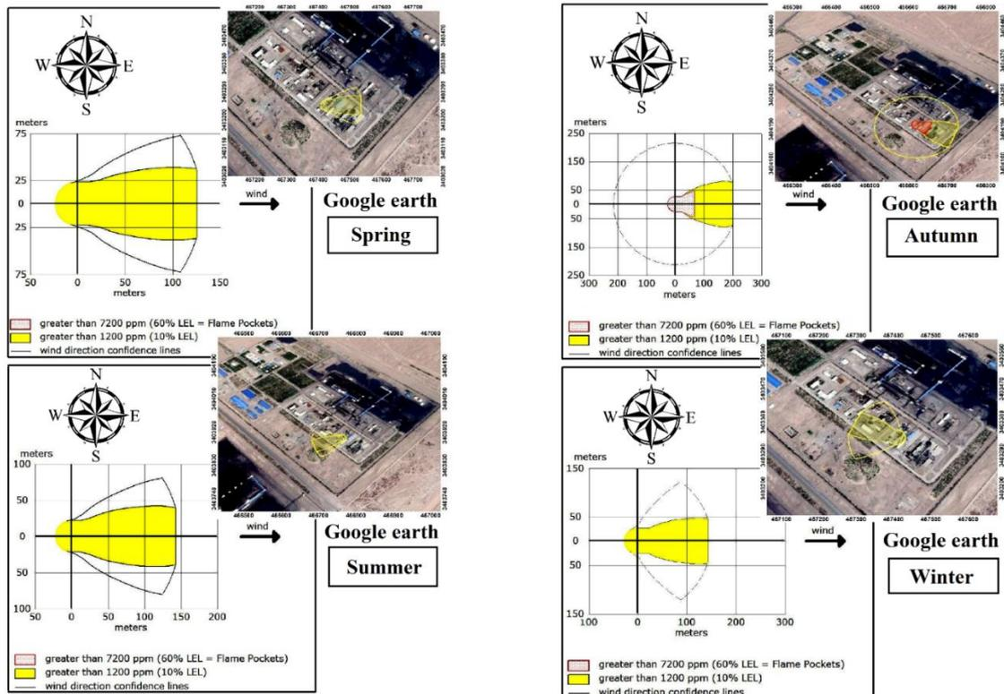
**Fig. 5. Graphical modeling of domain of formation of the benzene flammable vapor cloud at different distances from the tank in spring, summer, autumn and winter**
