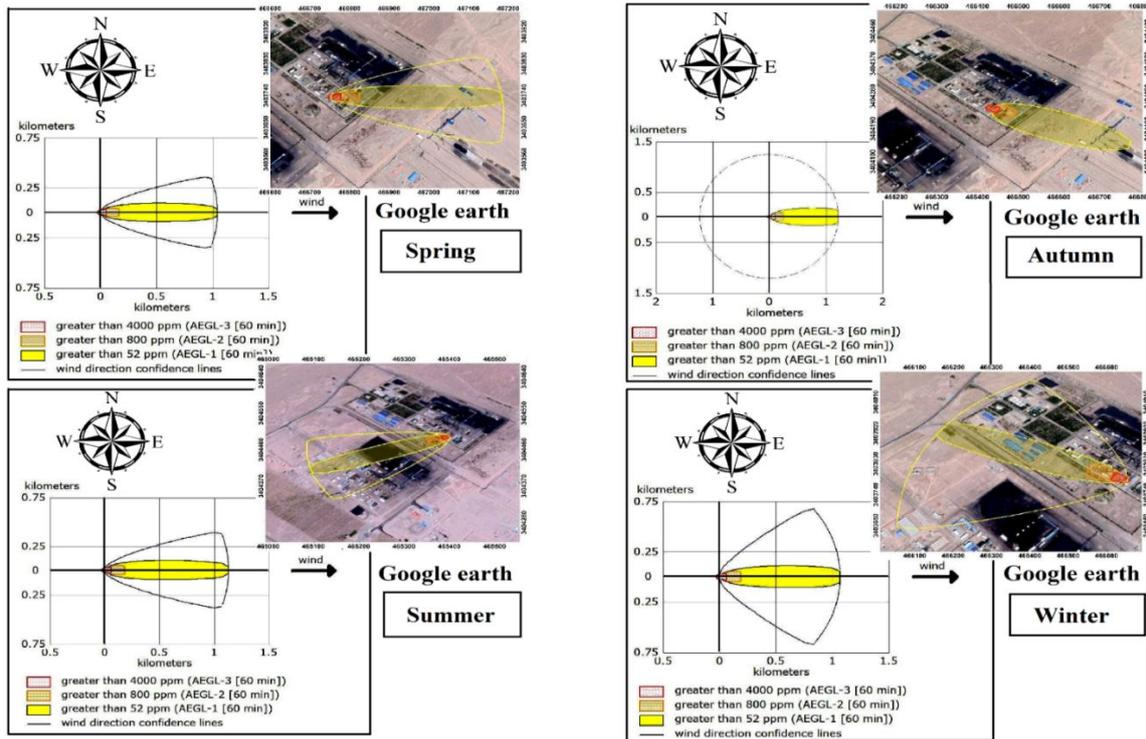
**Fig. 3. Graphical modeling of domain of formation of the benzene toxic vapor cloud at different distances from the tank in spring, summer, autumn and winter**
