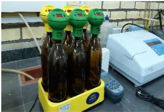
**Fig 2B.** Device for measuring BOD
