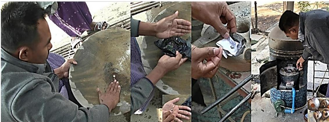
**Fig 3.** Gold refining process. This process took place on the street outside the gold shop. No protective attire, such as gloves or masks, were used during the whole process of amalgamation making and heating.
