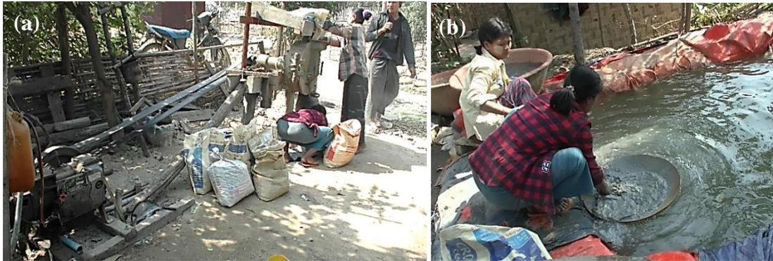
**Fig 2.** Ore crushing (a) and screening (b) process occurred in the yard. Ore crushing equipment, which is assembled from simple agricultural equipment, and reservoirs are distributed in courtyards with limited space. Among the people we interacted with, all family members who were able to work participated in ASGM activity for a household.
