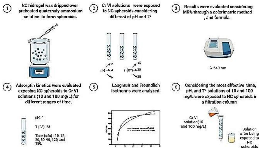
Fig 3. Cr VI removal process employing nanocellulose spheroids
