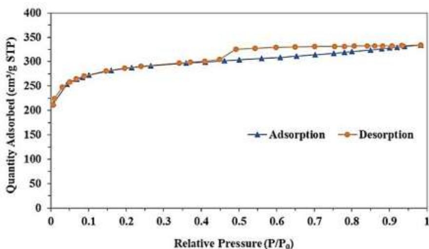
**Fig. 1.** Nitrogen adsorption-desorption isotherms of the optimal CCAC
