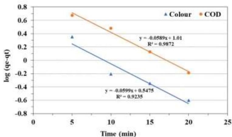
Fig. 11. Pseudo-first-order kinetic model for colour and COD adsorption
