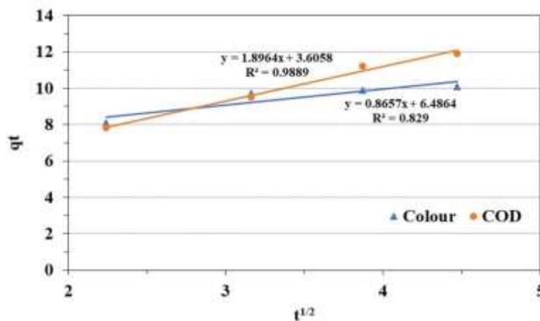
Fig. 13. Intraparticle diffusion model for colour and COD adsorption
