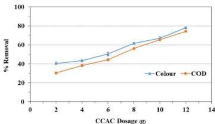
**Fig. 5.** The effect of the CCAC dosage on the removal efficiency
