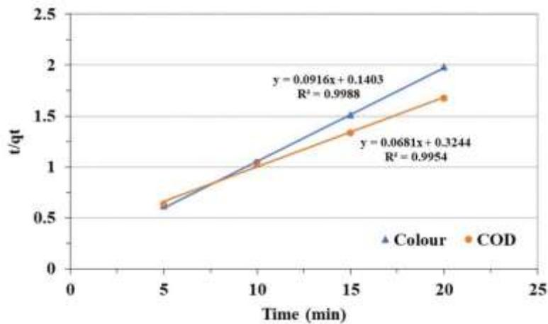
Fig. 12. Pseudo-second-order kinetic model for colour and COD adsorption
