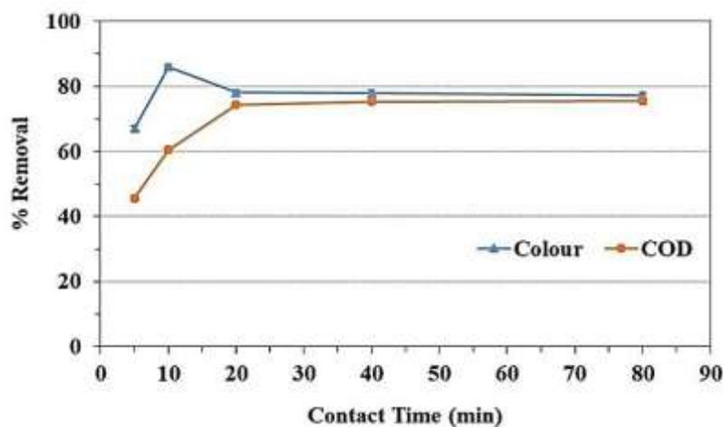
Fig. 7. The effect of the contact time on the removal efficiency
