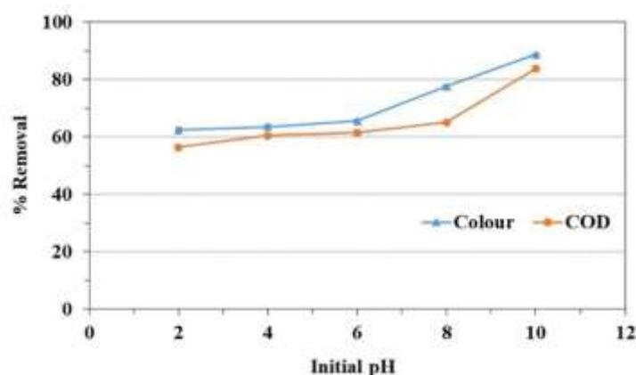
Fig. 9. The effect of the initial pH on the removal efficiency
