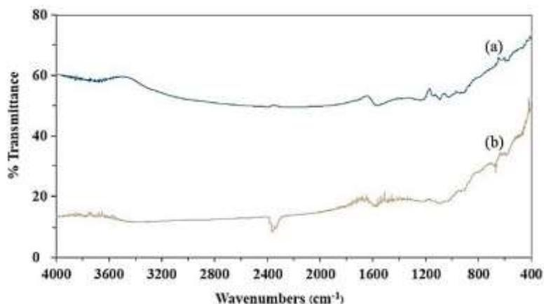
**Fig. 4.** FTIR spectra of the optimal CCAC (a) before adsorption and (b) after adsorption
