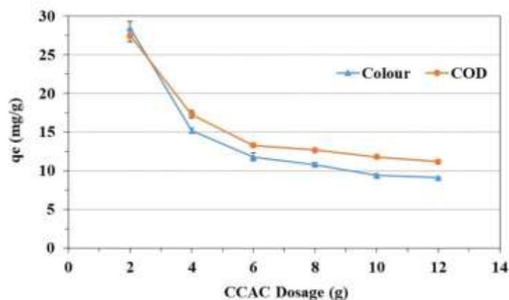
Fig. 6. The effect of the CCAC dosage on the adsorption capacity
