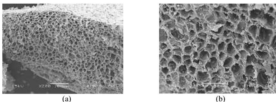
**Fig. 3.** SEM images of the optimal CCAC: (a) scale: 100  $\mu\text{m}$ , (b) scale: 50  $\mu\text{m}$
