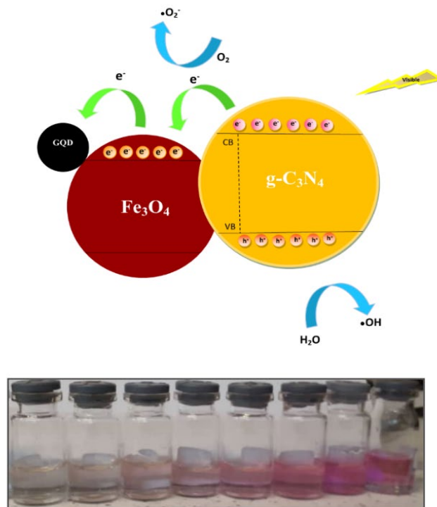
Fig. 9. proposed photocatalytic mechanism for degradation of RhB by (FGC) nanocomposite under visible light irradiation and degradation of RhB by (FGC) nanocomposite after 70 min.
