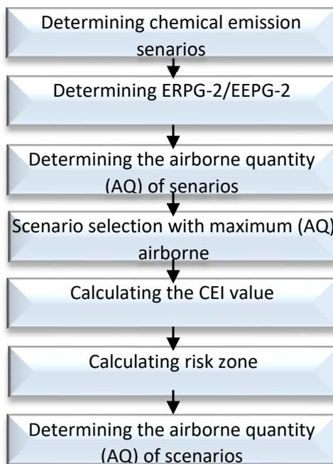
Fig. 3. Stages of implementation of the DOW Chemical Exposure Index (CEI) (Source: AIChE, 1998)
