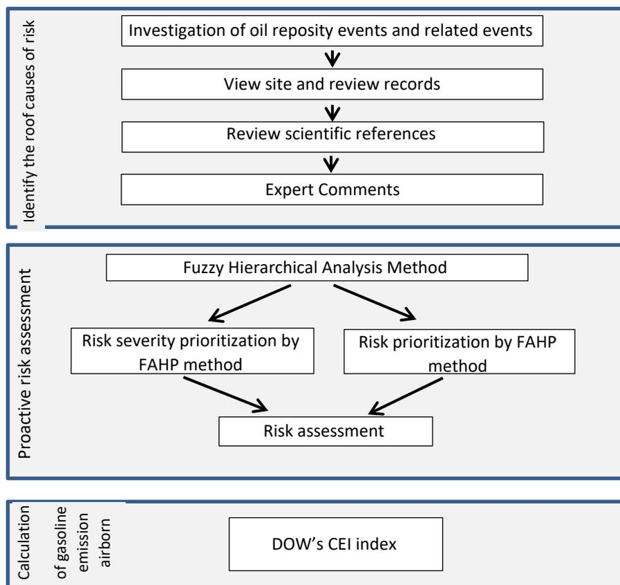
**Fig. 1.** The risk assessment process for toxic gases emission from the gasoline floating roof storage tank
