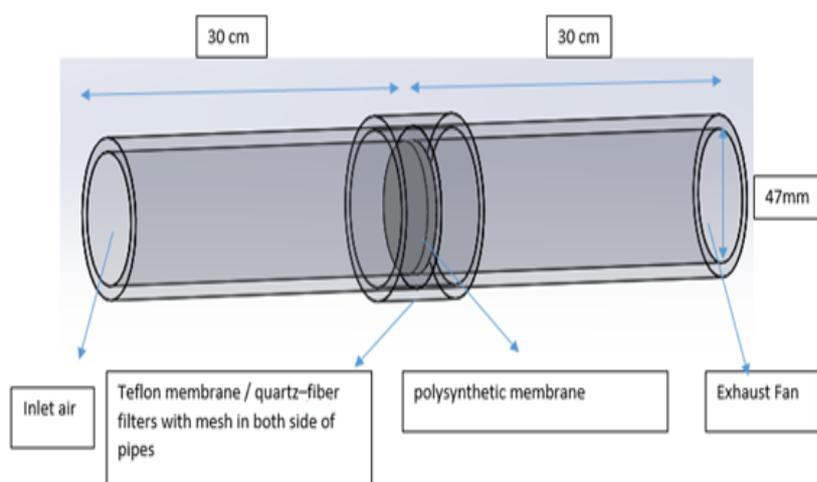
Fig 2. Schematic diagram of collecting PM.
