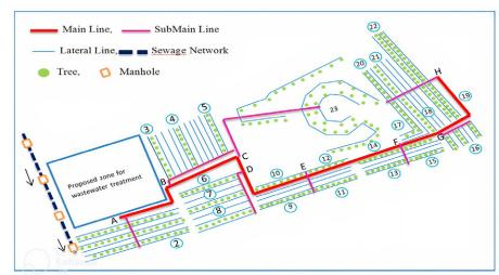
Fig 3. Layout of the proposed drip network for the garden of the new city of Ouled Djellal.
