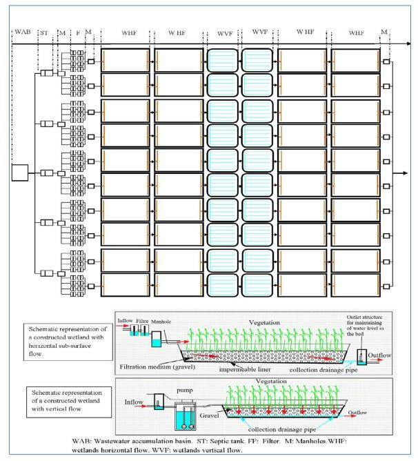
Fig 4. Design of a constructed wetlands system for wastewater treatment (HF-VF-HF).
