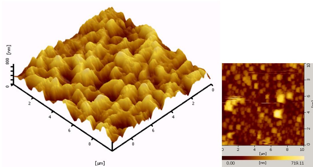
**Fig 10.** AFM images of composite flat sheet membrane (CFSM-1)
