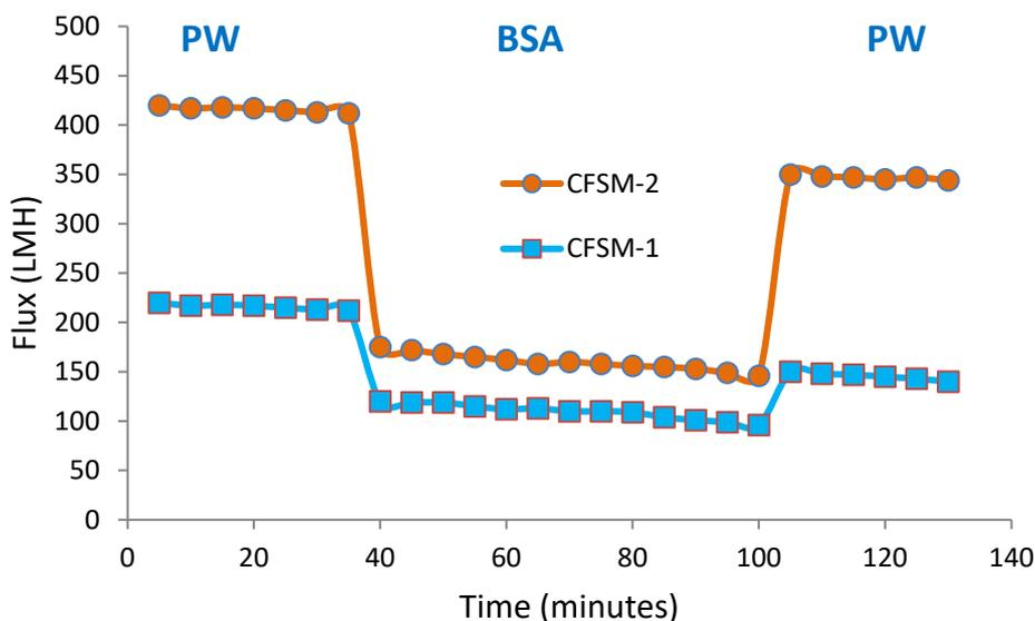
Fig 13. Fouling behavior of prepared membranes with filtration of DW & BSA solution (1000 mg/L, pH~7.4)
