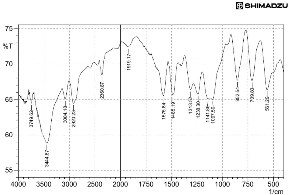
Fig 8. FTIR spectra of CFSM-1
