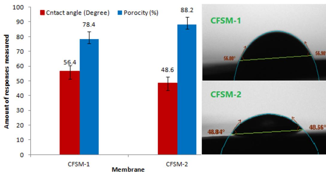
Fig 12. Static water contact angle and porosity of the composite membranes
