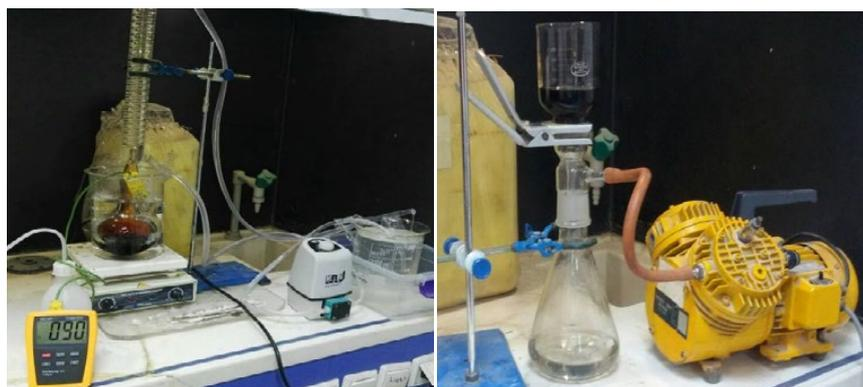
Fig 2. Preparation of the oxidized MWCNTs.
