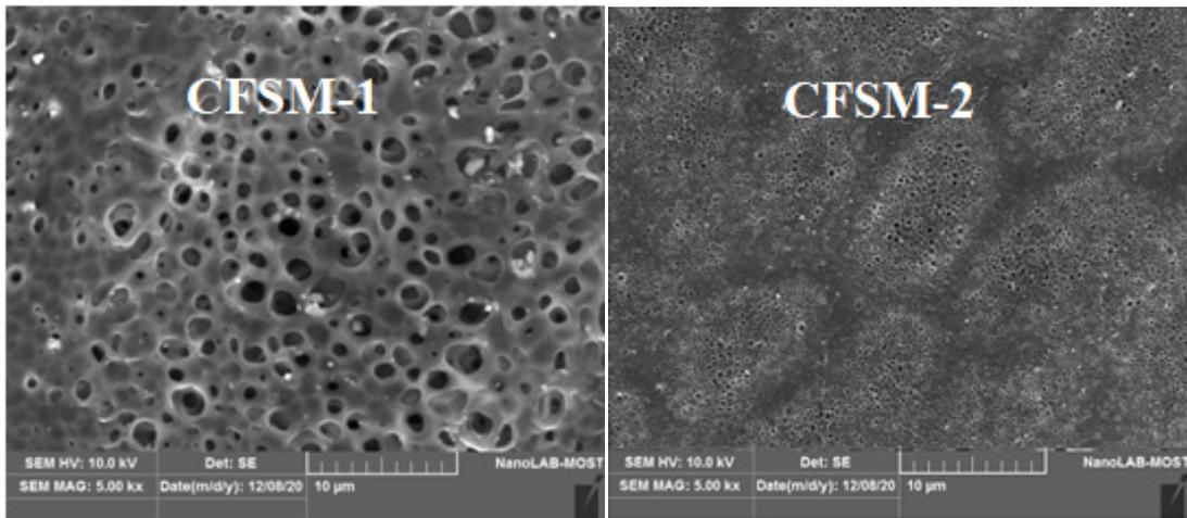
Fig 7. SEM images of composite flat sheet membranes with and without the nanomaterials.
