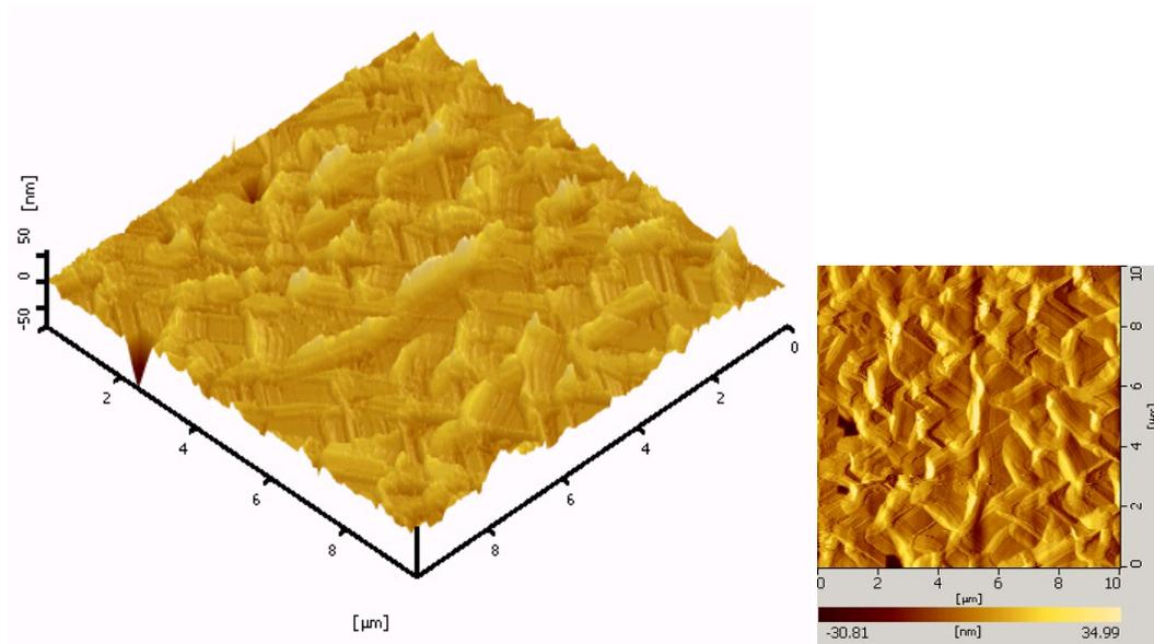
**Fig 11.** AFM images of composite flat sheet membrane (CFSM-2)
