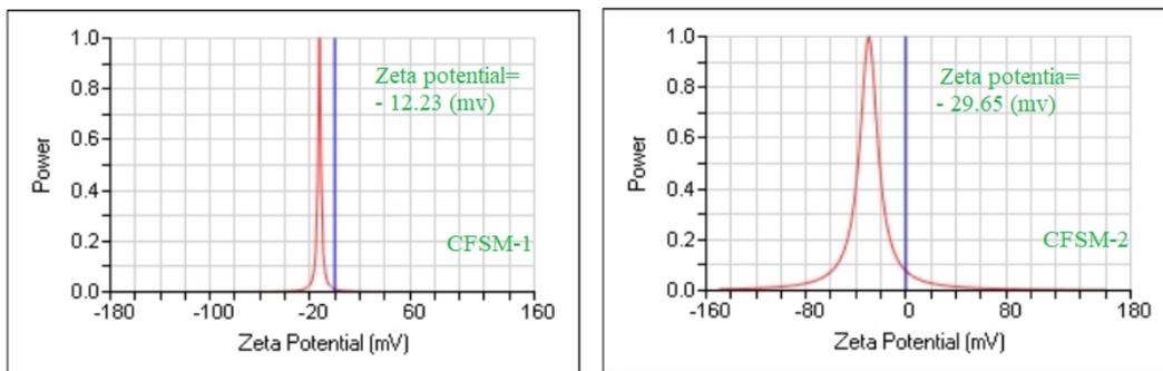
Fig 15. Zeta potential data for fabricated membranes (CFSM-1 and CFSM-2).
