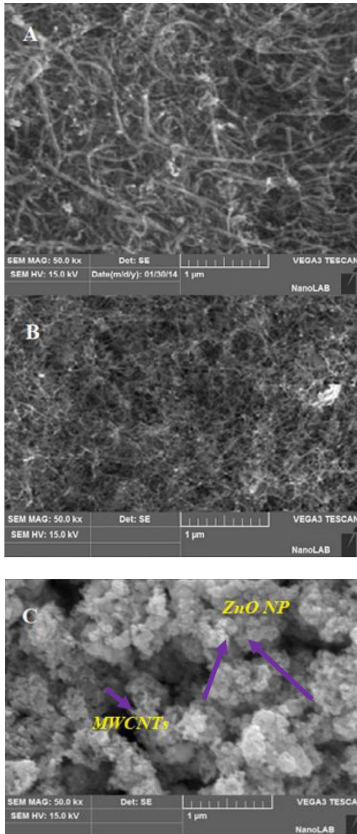
**Fig 6.** SEM images: (a) raw MWCNTs (b) oxidized MWCNTs and (c) OMCNTs/ZnO/AG
