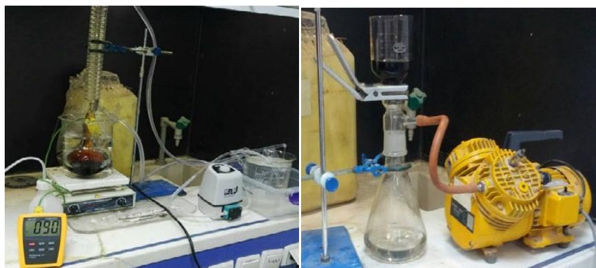
Fig 2. Preparation of the oxidized MWCNTs.
