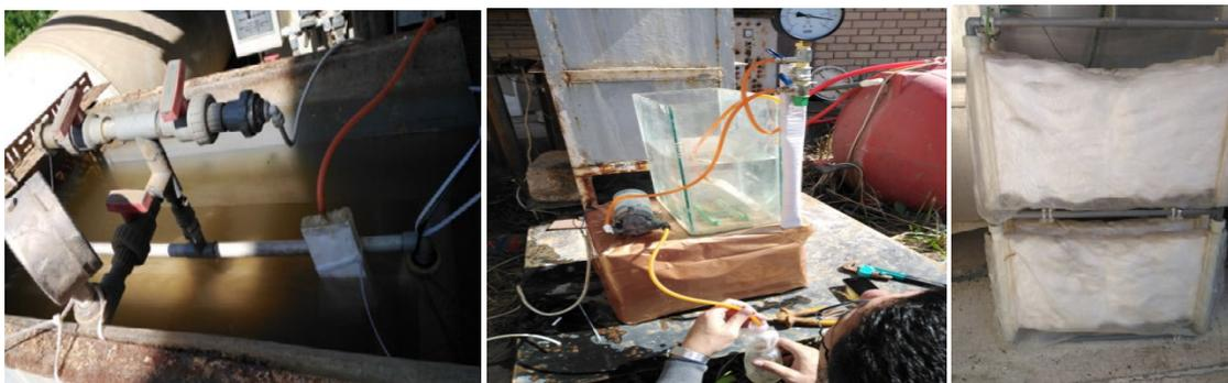
Fig 5. Our membrane operates within the MBR system of the Dairy factory of the College of Agriculture.
