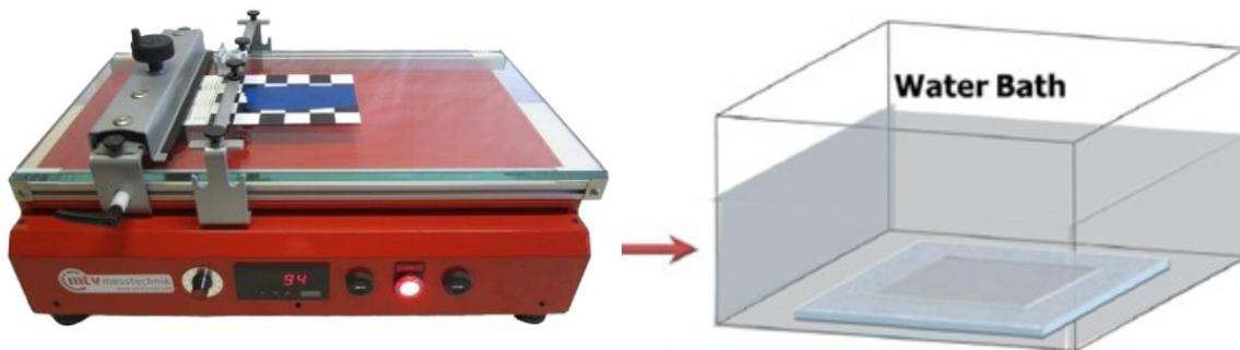
**Fig 3.** Phase inversion process for composite membranes fabrication using the motorized film applicator CX-4 (Germany)
