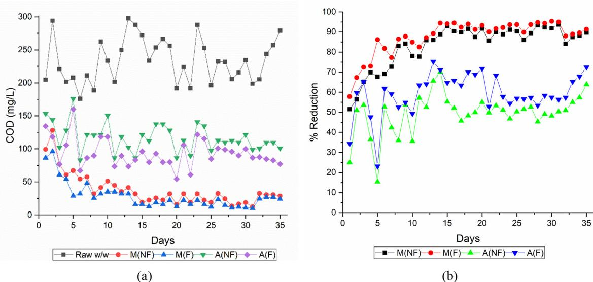
**Fig. 3.** Variation in (a) COD concentration and (b) Removal efficiency in microalgal and control system
