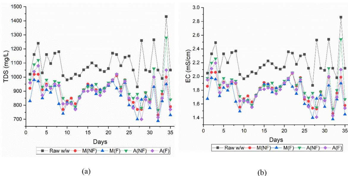
Fig. 8. Variation in (a) TDS and (b) EC concentration in influent and effluent
