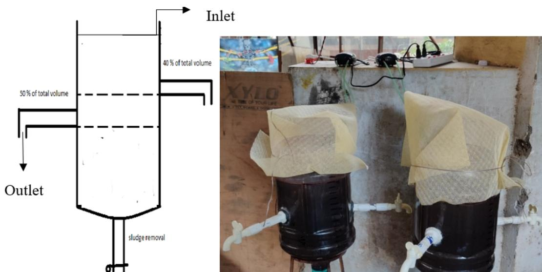
**Fig. 1.** Experimental setup of microalgal treatment for primary treated STP wastewater
