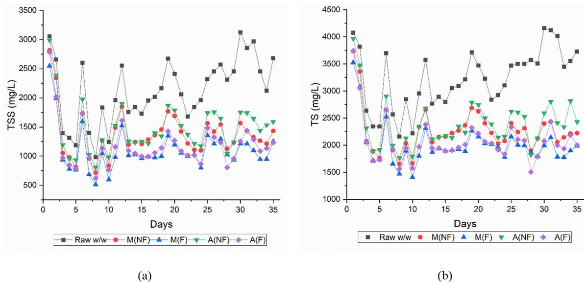
Fig. 7. Variation in (a) TSS and (b) TS concentration in influent and effluent
