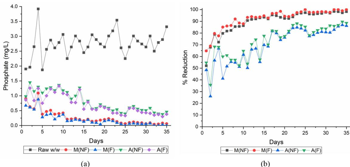
**Fig. 4.** Variation in (a) Phosphate concentration and (b) Removal efficiency in microalgal and control system
