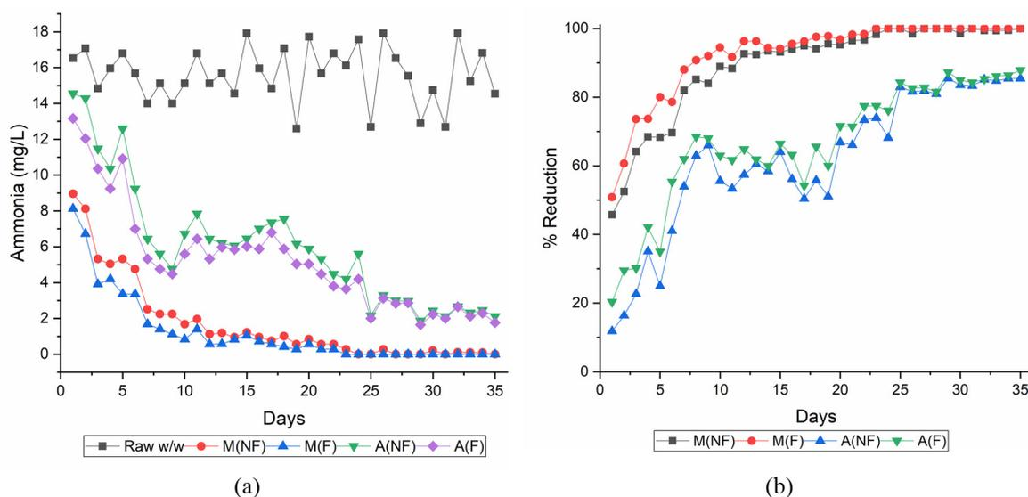
**Fig. 5.** Variation in (a) Ammonia concentration and (b) Removal efficiency in microalgal and control system
