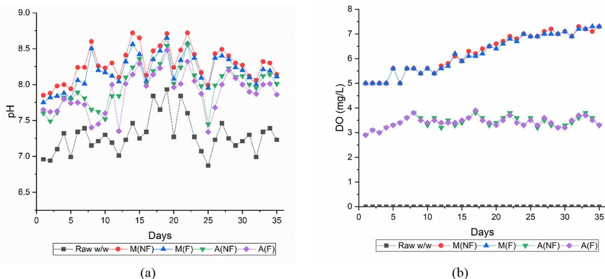
**Fig. 2.** Variation in (a) pH concentration and (b) DO concentration in influent and effluent
