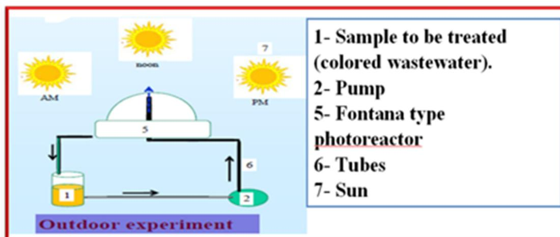
Fig 2. Schematic experimental diagram solar disinfection experiments
