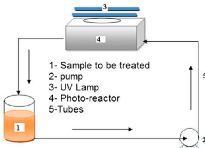
**Fig 1.** Photocatalytic reactor with artificial UV light
