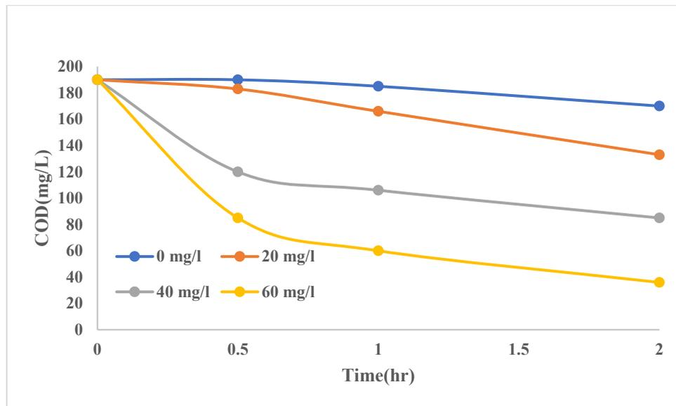
**Fig 4.** COD result with different concentration of TiO<sub>2</sub>
