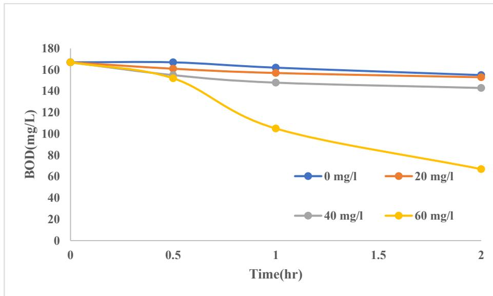
Fig 5. BOD result of sample with different concentration of TiO<sub>2</sub>
