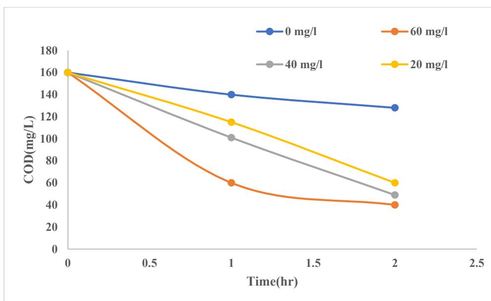
Fig 6. COD result of sample with different concentration of  $\text{TiO}_2$  with artificial UV light
