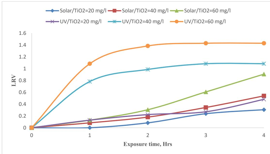
Fig 3. Effect of TiO<sub>2</sub> dosage on LRV of total coliforms
