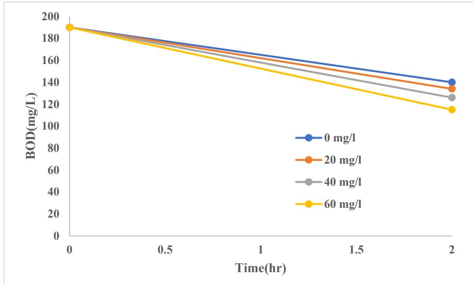
Fig 7. BOD result of sample with different concentration of TiO<sub>2</sub> with artificial UV light
