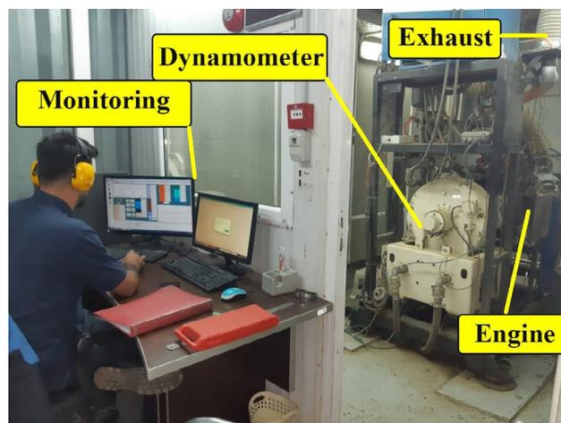
Fig. 1. Used experimental setup
