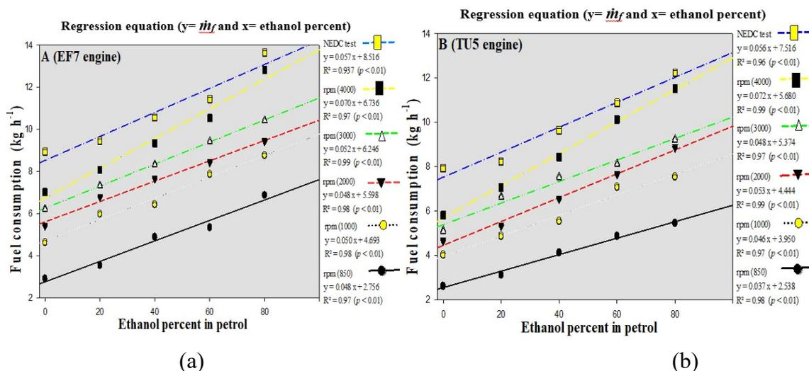
**Fig. 3.** The positive linear regression model for predicting the fuel consumption trait ( $\dot{m}_f$ ) under the interaction between add ethanol (from 0 to 80%) to gasoline (0, 20, 40, 60 and 80 %) and engine speeds (850, 1000, 2000, 3000 and 4000 rpm along with the NEDC test) in the (a)- EF7 and (b)- TU5 engines.
