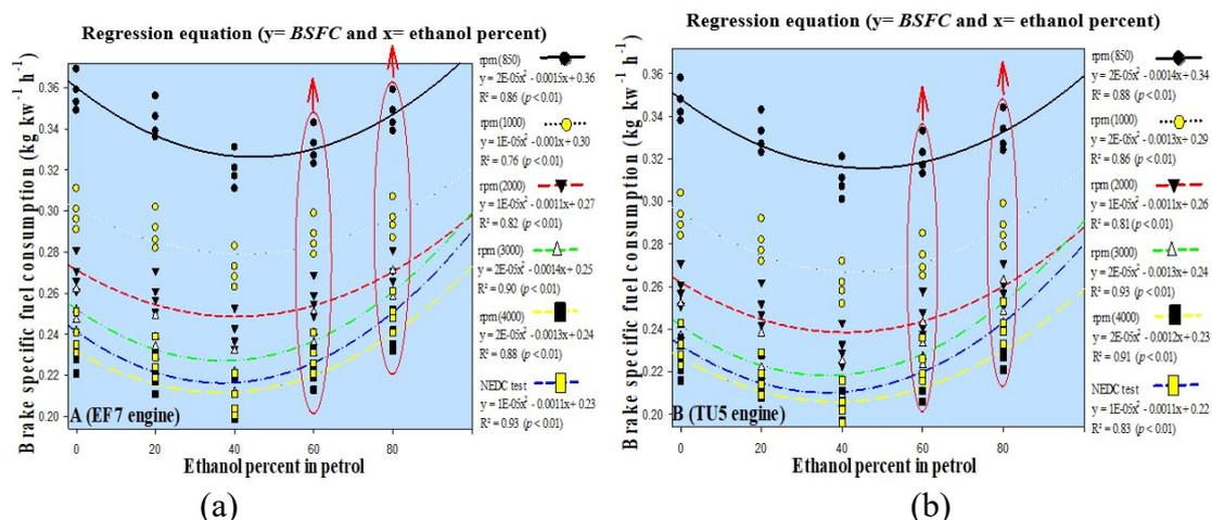
**Fig. 5.** Positive second-order polynomial regression model for predicting the brake specific fuel consumption trait (BSFC) under the interaction between add ethanol (from 0 to 80%) to gasoline and engine speeds (850, 1000, 2000, 3000 and 4000 rpm along with the NEDC test) (a)-in the EF7 and (b)- in the TU5 engines.
