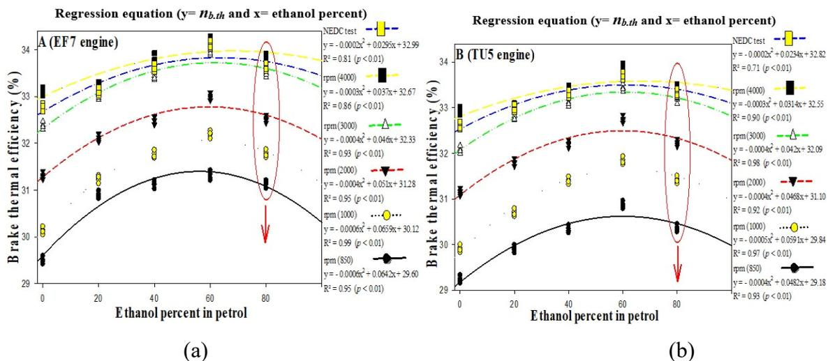
**Fig. 4.** The negative second-order polynomial regression model for predicting the brake thermal efficiency character ( $n_{b,th}$ ) under the interaction between add ethanol (from 0 to 80%) to gasoline and engine speeds (850, 1000, 2000, 3000 and 4000 rpm along with the NEDC test) (a)- in the EF7 and (b) in the TU5 engines.
