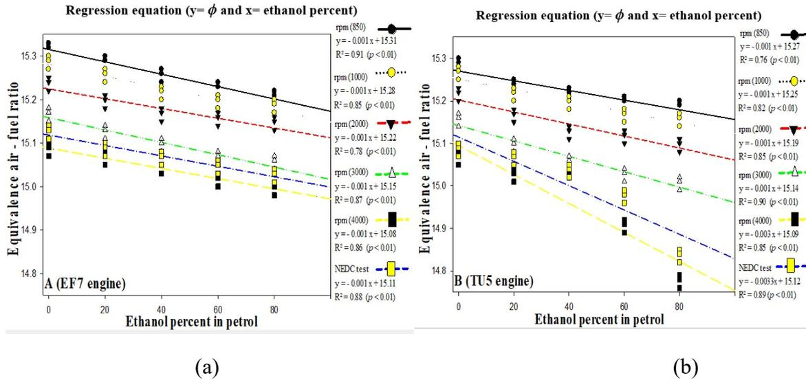
**Fig. 2.** The negative linear regression model for predicting the equivalence air-fuel ratio trait ( $\phi$ ) under the interaction between add ethanol (from 0 to 80%) to gasoline and engine speeds (850, 1000, 2000, 3000 and 4000 rpm along with the NEDC test) (a)-in the EF7 and (b)- in the TU5 engines.
