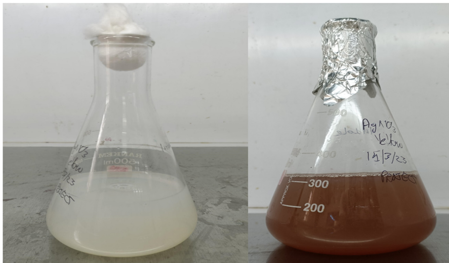
Fig. 1. Color change of silver nitrate solution due to biosynthesis of silver nanoparticles.
