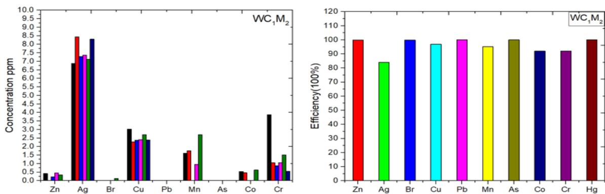
**Fig. 8.** Ratio of post-treatment concentrations and efficiency ratio for sample WC<sub>1</sub>M<sub>2</sub>
