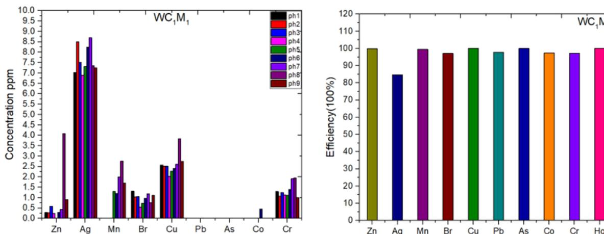
Fig. 11. Post-treatment elements concentrations and treatment efficiency percentage in sample WC<sub>1</sub>M<sub>1</sub>
