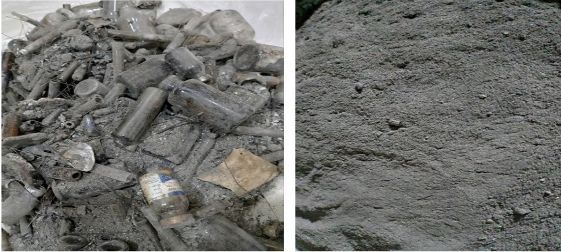
Fig. 1. Medical waste ash before and after the grinding process
