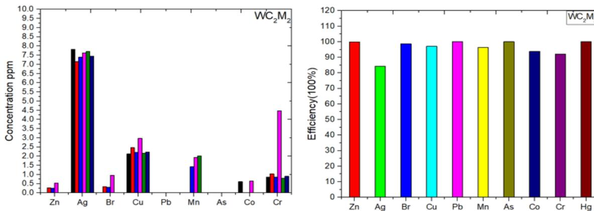
Fig. 10. Ratio of post-treatment concentrations and efficiency ratio for sample WC<sub>2</sub>M<sub>2</sub>
