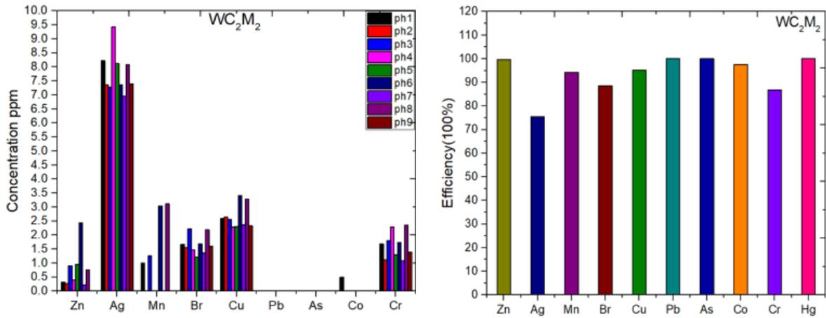
Fig. 14. Post-treatment elements concentrations and treatment efficiency percentage in sample WC<sub>2</sub>M<sub>2</sub>
