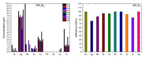
Fig. 12. Post-treatment elements concentrations and treatment efficiency percentage in sample WC<sub>1</sub>M<sub>2</sub>
