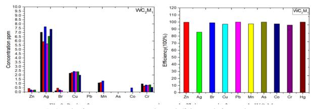
Fig. 9. Ratio of post-treatment concentrations and efficiency ratio for sample WC<sub>2</sub>M<sub>1</sub>
