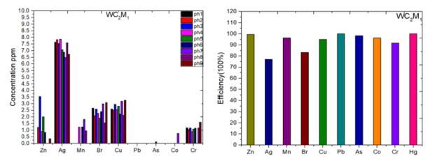
Fig. 13. Post-treatment elements concentrations and treatment efficiency percentage in sample WC<sub>2</sub>M<sub>1</sub>
