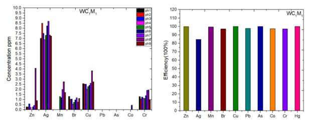
Fig. 11. Post-treatment elements concentrations and treatment efficiency percentage in sample WC<sub>1</sub>M<sub>1</sub>
