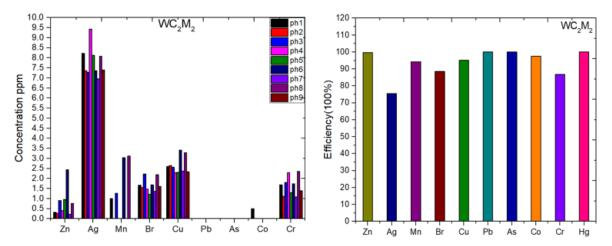
Fig. 14. Post-treatment elements concentrations and treatment efficiency percentage in sample WC, M,
