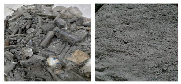
Fig. 1. Medical waste ash before and after the grinding process
