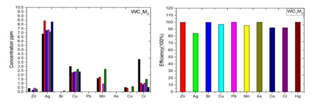
Fig. 8. Ratio of post-treatment concentrations and efficiency ratio for sample  $WC_1M_2$
