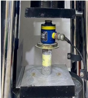
Fig. 5. Concrete pattern when using pistons to measure resistance.
